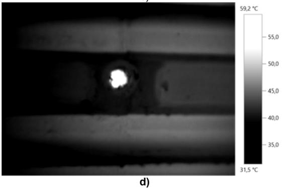
Fig. 4. The thermal images of IM defects with explicit manifestation:
