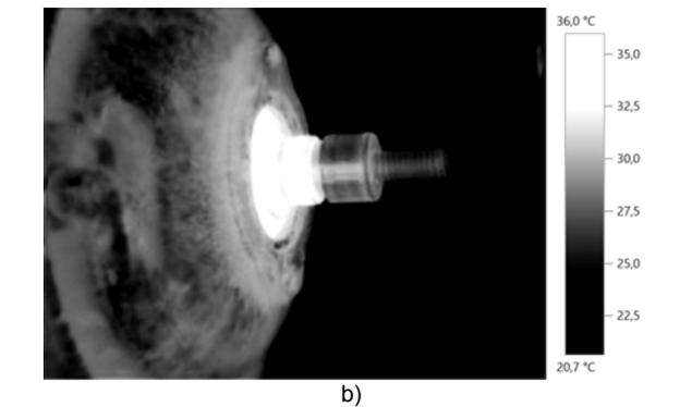
Fig. 2. The thermal images of the defects of IM front bearing: with a shut bearing cap; b) with an open bearing cap
