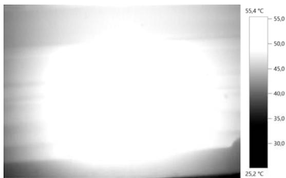
Fig. 3. The thermal image manifestation of IM stator core overheat
