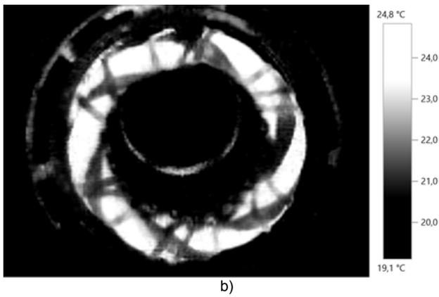
Fig. 1. The determination of the time constants of the stator winding heating and cooling: a) a partially heated winding; b) a partially cooled winding
