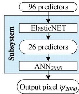
Fig.4. Model of elastic net + ANN hybrid subsystem dedicated to a single pixel  $\psi_{2000}$
