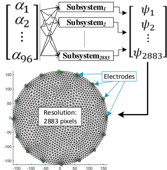
Fig.3. Model of the ECT system converting electrical signals into 2D image of cross-section
