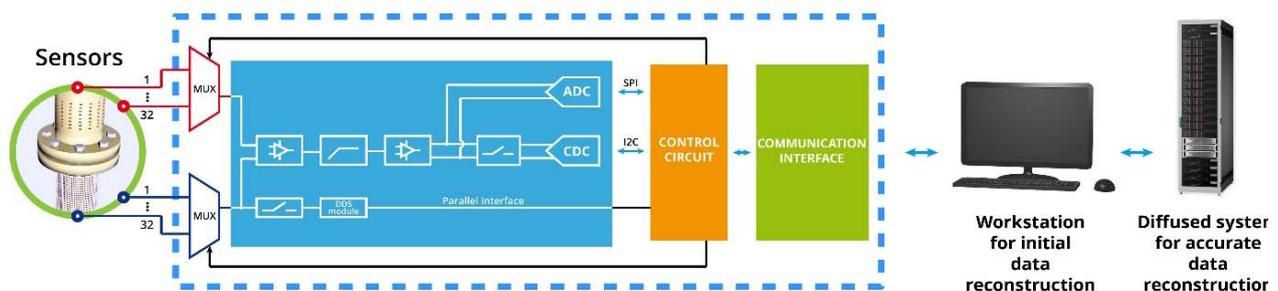
Fig.1 Schematic model of Smart ECT measurement system
