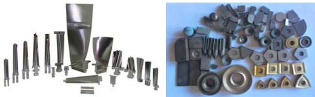
Fig. 8 – The parts of the gas turbine engines and cutting tools of powder materials obtained by the new technology.
