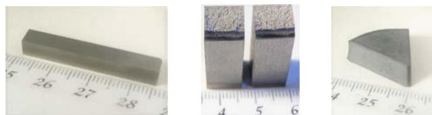
Fig. 1. Samples from powder materials after preliminary sintering
