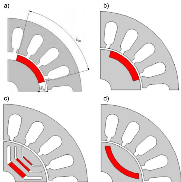
Fig. 1. Selected structures of PM synchronous motor
