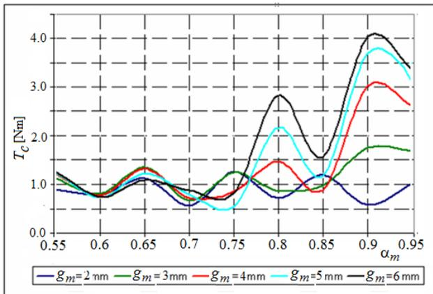
Fig. 5. Impact of the design variables on the cogging torque
