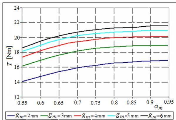
Fig. 3. Impact of the design variables on the electromagnetic torque
