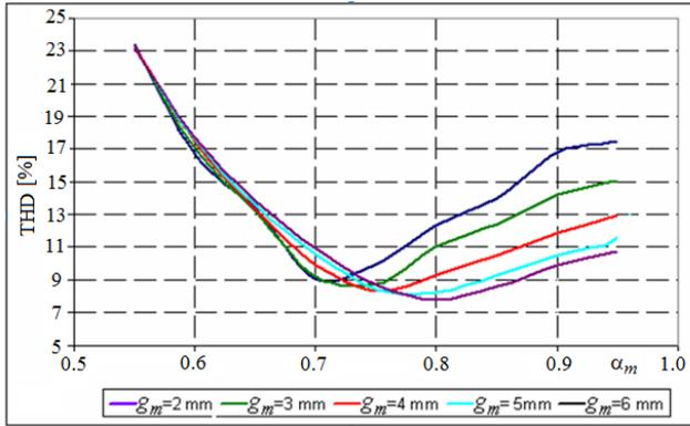
Fig. 4. Impact of the design variables on THD coefficient
