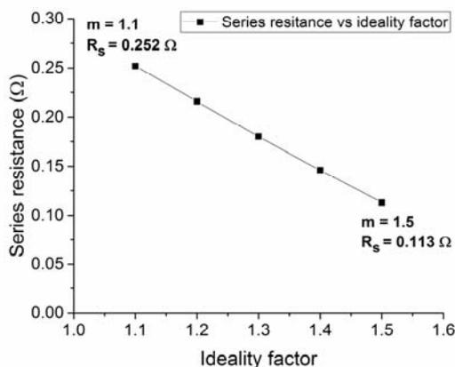
Fig.2. (a) Variation of resistance series  $R_s$
