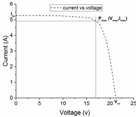
Fig.2. The I-V curve of a solar panel
