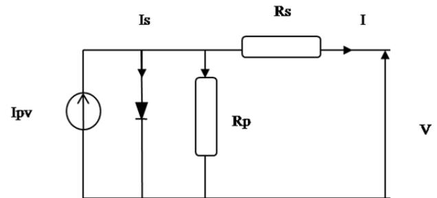
Fig.1. Single diode model of solar cell
