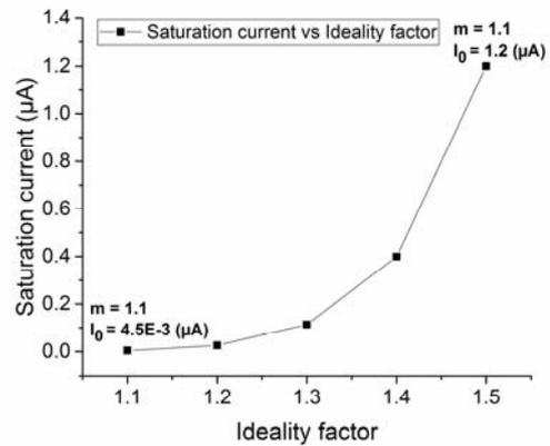
Fig.2. (c): Variation of the saturation current  $I_0$
