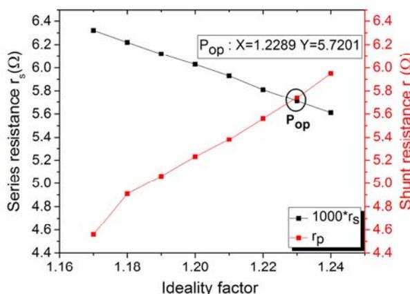
Fig.4. Exact graphical determination of the Pop point
