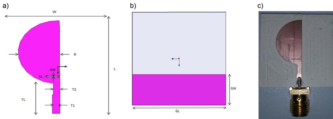
Fig.1: Proposed UWB antenna. (a) Front View (b) Ground Plane (c) Fabricated Antenna (Picture Not up to Scale)
