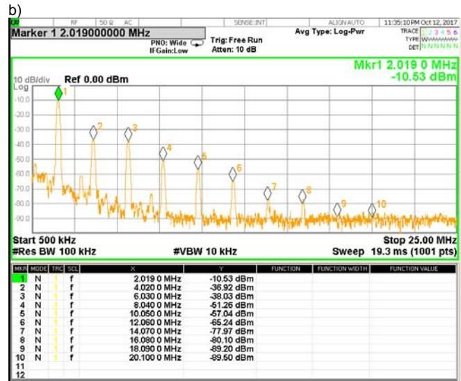
Fig.8. Sinusoidal output signal with 2.01MHz frequency (a) sinusoidal waveform (b) frequency spectrum and harmonics
