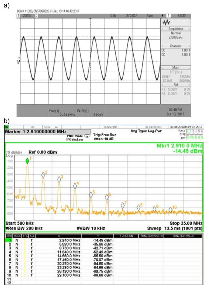
Fig.9. Sinusoidal output signal with 2.91MHz frequency (a) sinusoidal waveform (b) frequency spectrum and harmonics
