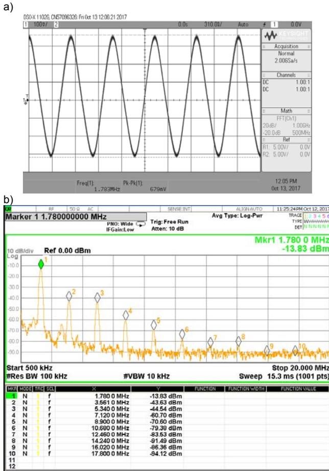
Fig.7. Sinusoidal output signal with 1.78MHz frequency (a) sinusoidal waveform (b) frequency spectrum and harmonics
