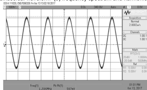
Fig.5. Sinusoidal waveform with 1.59MHz frequency
