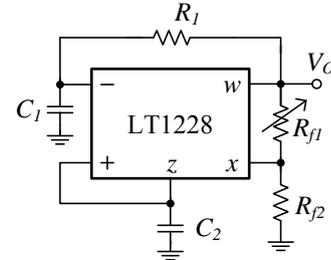
Fig.2. Proposed sinusoidal oscillator
