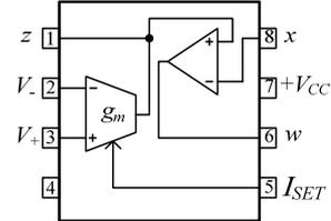
Fig.1. Detail of LT1228 (a) electrical symbol (b) equivalent circuit (c) pin configuration
