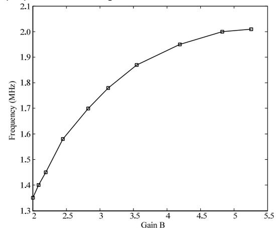
Fig.6. Oscillation Frequency when varying gain  $B$
