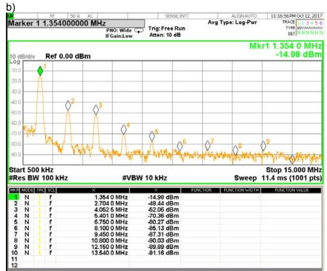
Fig.4. Sinusoidal output signal with 1.35MHz frequency (a) sinusoidal waveform (b) frequency spectrum and harmonics
