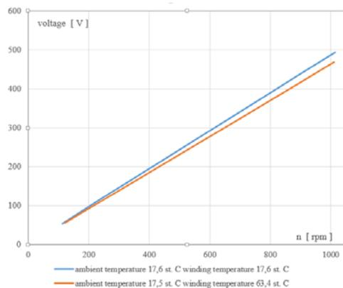
Fig. 10. The dependence of output voltage on rotational speed
