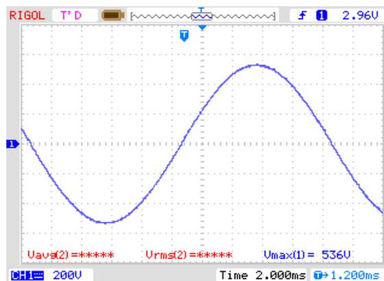
Fig. 11. The waveform of line-to-line voltage for the generator at idle
