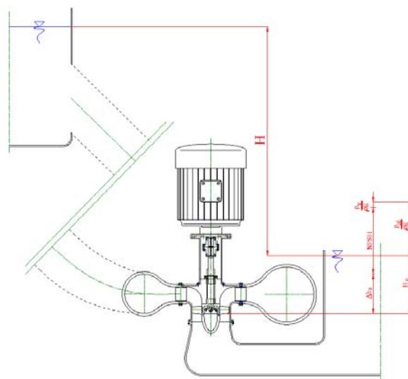
Fig. 1b Set-up of hydro generator - source of supply above turbine
