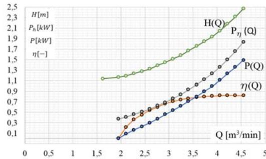
Fig. 6. Characteristics of the tested pico turbine elaborated on the basis of Best Efficiency Point parameters
