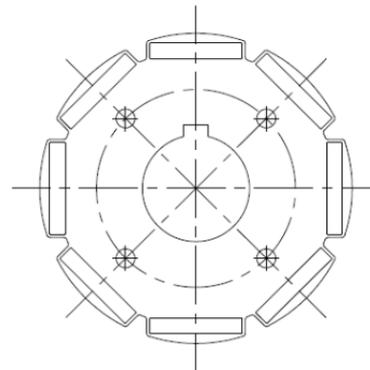
Fig. 7. The shape of rotor's sheet
