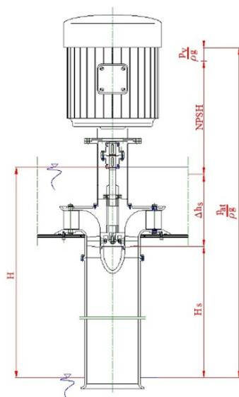
Fig. 1a Set-up of hydro generator - source of supply below turbine
