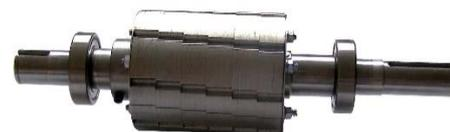
Fig. 8. View of the generator rotor with slanted magnets.
