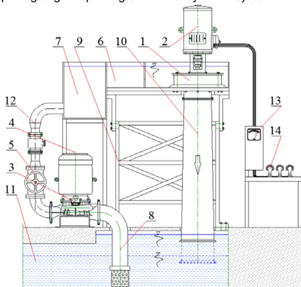
Fig. 4. Water pico turbine and three-phase generator test stand. 1 - turbine, 2 - generator, 3 - supplying pump, 4 - pump motor, 5 - valve, 6 - inflow channel, 7 - buffer, 8 - suction pipe, 9 - load bearing construction, 10 - draft tube of the turbine, 11 - underfloor tank, 12 - discharge pipeline, 13 - electrical meter, 14 - electrical resistor
