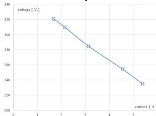
Fig. 12. The dependence of output voltage on load current
