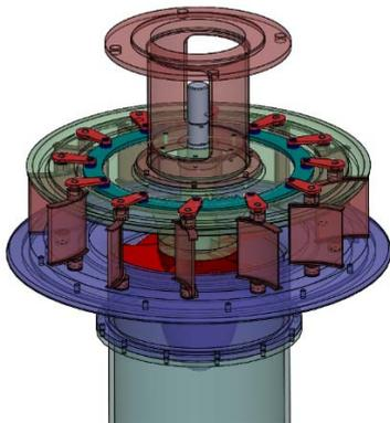
Fig.3. 3D Turbine with a four-blade rotor
