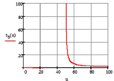
Fig.5e. Dependence of the block operating time  $t_b$  from the productivity of the general block  $u_n=55$  with respect to the size of the buffer  $B_{max}=50$  of the general block  $p_n=50$
