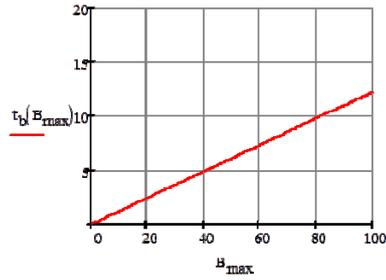
Fig.5c. Dependence of the time of permanence on buffer size for the performance of the block  $p=45$  and the productivities of the general block  $u_n=55$
