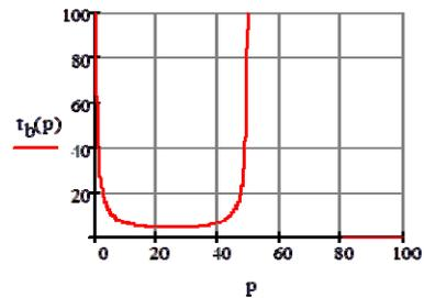
Fig.5d. Dependence of the time of permanence on buffer  $t_b$  from the performance of the block  $p_n$  and the productivities of the general block  $u_n=55$
