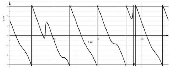
Fig.4. Phase-frequency characteristic of the total signal for three measurement objects with different reflection coefficients
