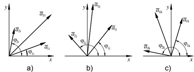
Fig. 2 Vector diagrams of signals reflected from two objects and the total signal on the  $i$ -th (a),  $j$ -th (b) and  $k$ -th (in) frequencies
