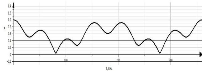
Fig.3. Amplitude-frequency characteristic of the total signal for three measurement objects with different reflection coefficients
