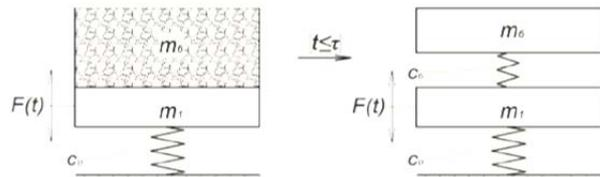
Fig. 1. Change from the combined discrete-continuous mathematical model (a) to a discrete mathematical model (b)
