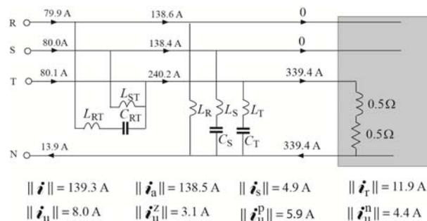
Fig. 8. Results of compensation with a reduced complexity compensator.
