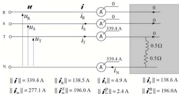
Fig. 6. Example of an unbalanced load and its analysis.
