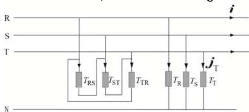
Fig. 2. A structure of reactive compensator.
