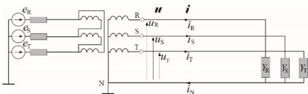
Fig. 1. A four-wire system with fictitious single-phase loads.
