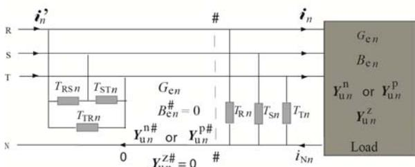
Fig. 3. Load with reactive compensator for the  $n^{\text{th}}$  order harmonic of the positive or negative sequence.
