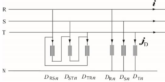
Fig. 5. A compensator with branches of reduced complexity and  $D_n$  susceptance.
