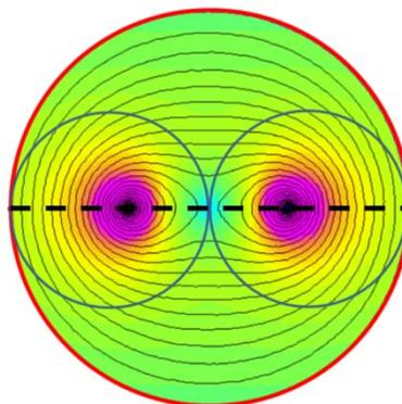
Fig. 14. Magnetic field distribution for two parallel wires with symmetrical current and with arbelos graph.
