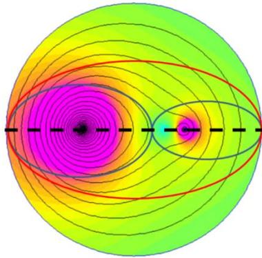
Fig.15. Magnetic field distribution for two parallel wires with asymmetrical current and arbelos graph.
