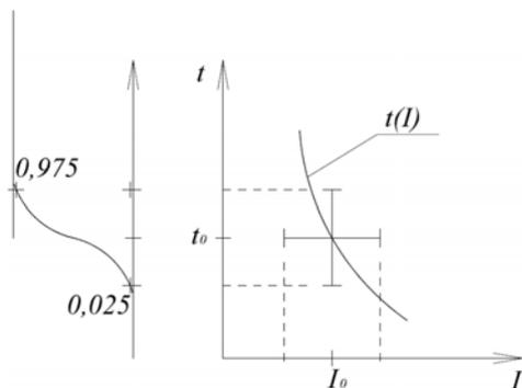
Fig. 2. The time-current characteristic of a fuse and its statistical description of uncertainty for assumed confidence level 0,95
