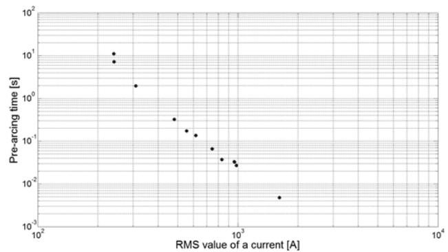
Fig. 4. Time-current characteristic for 63 A MV fuses
