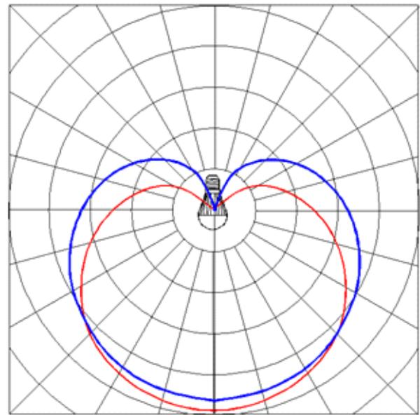
Fig. 5. Surface profile with constant luminance (blue curve) against the luminous intensity distribution of the LED with a diffusing semidome (red curve).
