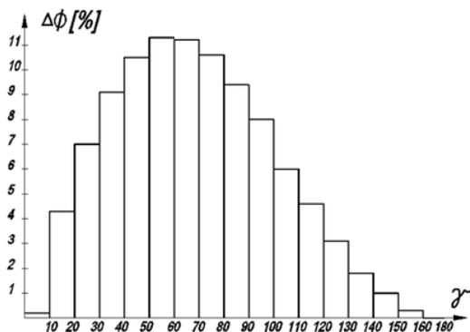
Fig. 2. Distribution of the luminous flux of the LED, with a semidome shaped luminous block, in equal, 10-degree compartments of the flat angle  $\Delta\gamma$ .
