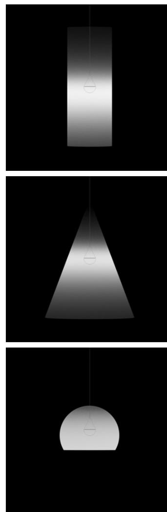
Fig. 3. Calculated distribution of luminance on the surface of milk shades, with scattering LED with semi-spherical dome application. As can be seen from Figure 3, the consequence of using a LED with semi-spherical dome is the specific distribution of luminance on the surface of the lampshade with relatively small bright area of the lampshade. It extends in a range from the light output opening, more or less to the height of the source attachment. Going up, this area continues to
