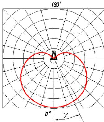
Fig. 1. LED with a diffusing semidome and its luminous intensity distribution.
