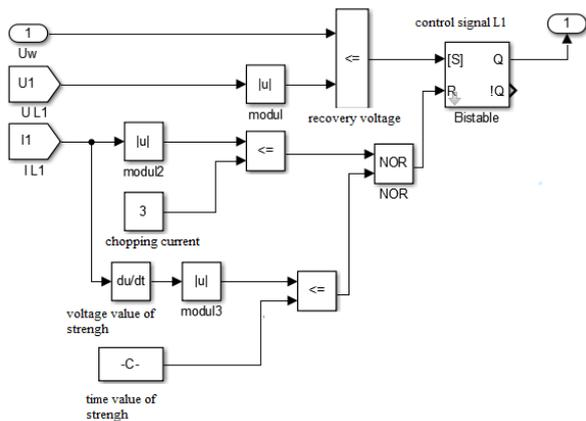
Fig.3 Voltage and current conditions for controlling the pole of a circuit breaker
