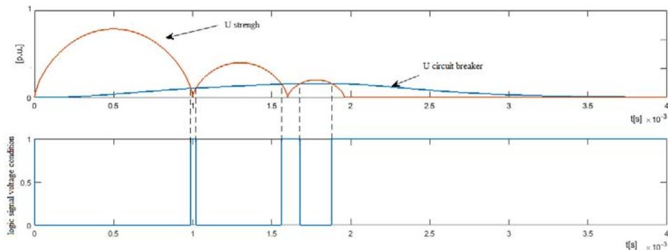
Fig. 7 Scheme of operation of the voltage element of the algorithm that generates the signal that controls the poles of the circuit breaker
