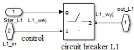
Fig.1 Scheme of one of the poles of a circuit breaker
