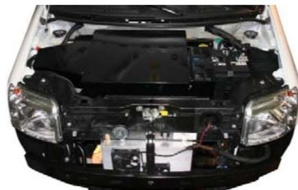
Fig. 4. View of the Fiat Panda EV engine compartment with electric drive system.
