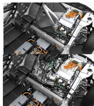
Fig. 1. Comparison of BMW i3 powertrains without REX and with REX [4].
