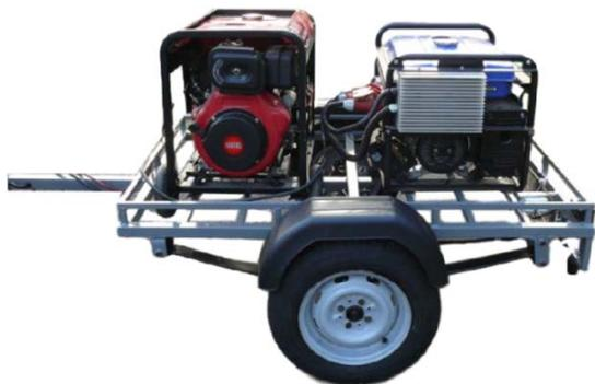
Fig. 6. Trailer with a Range Extender System.
