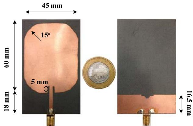
Fig. 1: Built prototype of the multiband antenna.
