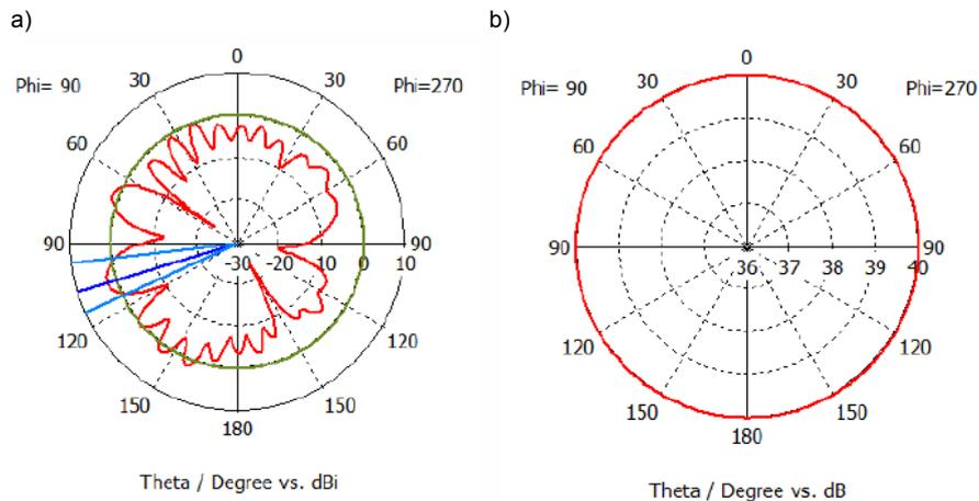
Fig. 5: 26 GHz (5G) Radiation Diagram. (a) E Plan, (b) H Plan.
