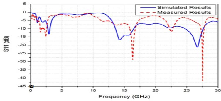
Fig. 2: The S11 parameter of the proposed antenna.
