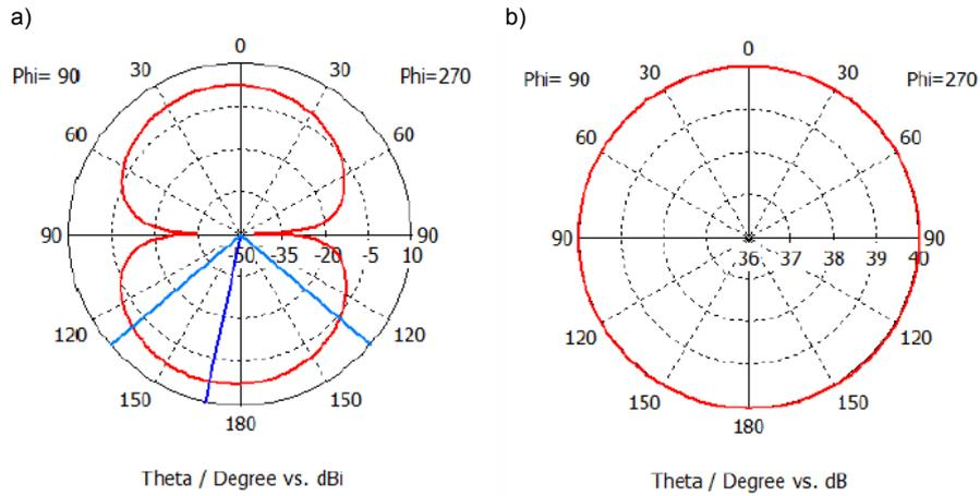
Fig. 3: 1575 MHz (GPS) radiation diagram. (a) E Plan, (b) H Plan
