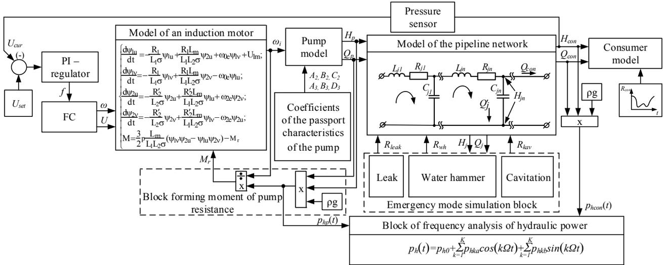
Fig.1. The block diagram of the model of the system of the automatic control of the pump variable-frequency electric drive
