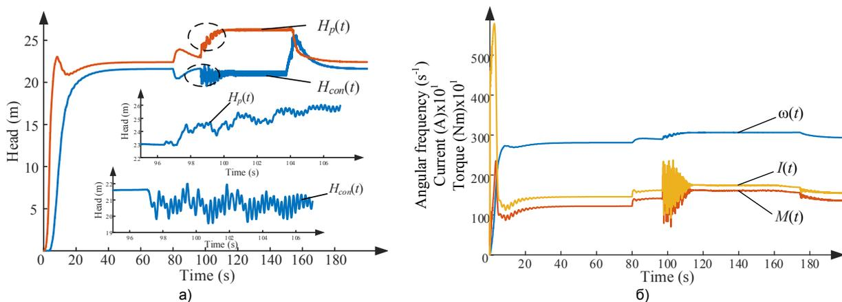
Fig.4. The curves representing the alteration of technological (a) and electromechanical (b) parameters of PC at the occurrence of cavitation in the hydronetwork
