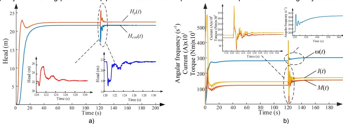
Fig.2. The curves representing the alteration of technological (a) and electromechanical (b) parameters of PC at the occurrence of a leakage in the pipeline network at time moment  $t=120$  s
