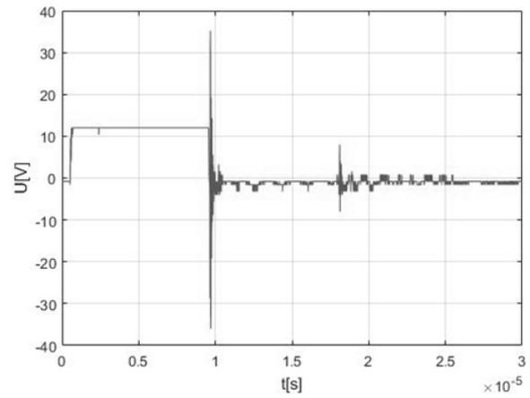
Fig. 12 The voltage waveform at the gate of the transistor ( $U_{gs}$ ) as a function of time – no brake down on the spark gap
