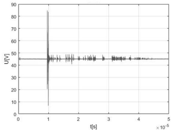
Fig. 14. The voltage waveform on the main capacitor of the HV triggering system ( $U_{zas}$ ) as a function of time - brake down on the spark gap
