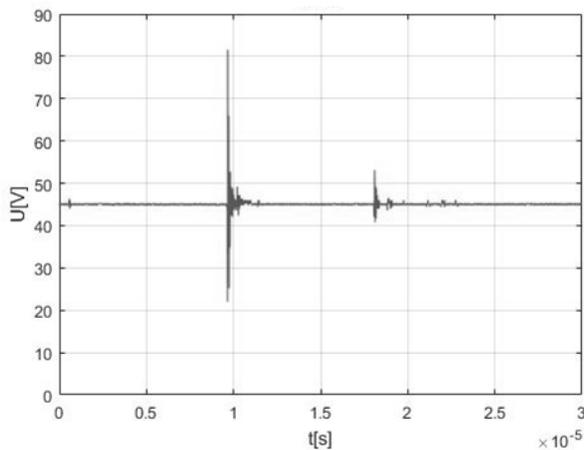
Fig. 10. Voltage waveform ( $U_{zas}$ ) on the main capacitor of the HV trigger unit as a function of time – no spark on the spark gap
