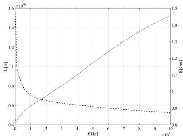
Fig. 7. The results of the measurement of inductance and resistance of the primary winding as a function of frequency (secondary winding shorted, “-” – resistance, “- -” – inductance)
