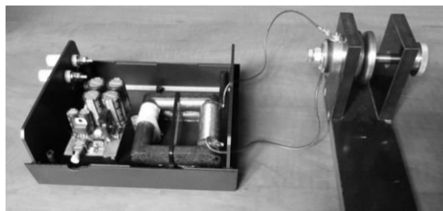
Fig. 3 HV trigger with a three-electrode spark gap
