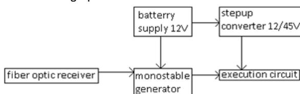
Fig. 1 The basic block diagram of the HV trigger unit
