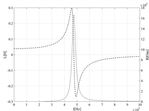
Fig. 6. The results of the measurement of inductance and resistance of the secondary winding as a function of frequency (secondary winding opened, “-” – resistance, “- -” – inductance)
