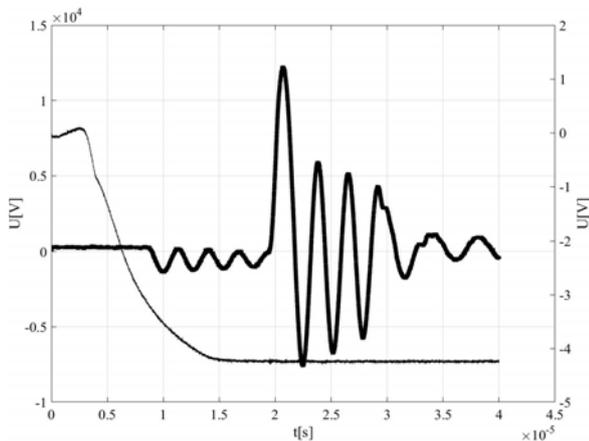
Fig. 18. Voltage waveform at the HV trigger output ( $U_{wy}$ ) – brake down on the spark gap
