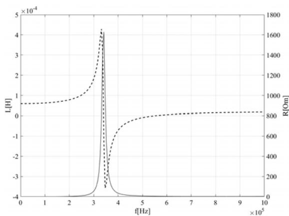
Fig. 5. The results of the measurement of inductance and resistance of the primary winding as a function of frequency (secondary winding opened, “-” – resistance, “- -” – inductance)
