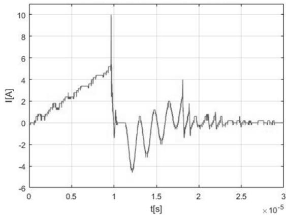
Fig. 9. Current waveform ( $I_{zas}$ ) as a function of time in the main execution circuit of the HV release system – no brake down on the spark gap
