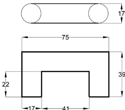
Fig. 4. Geometric dimensions of the ferrite core used for the construction of the pulse transformer (all dimension are given in mm)
