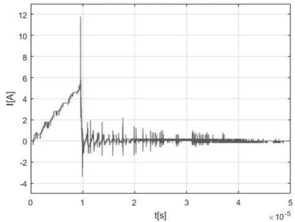
Fig. 13. The current waveform ( $I_{zas}$ ) as a function of time in the main execution circuit of the HV triggering system - brake down on the spark gap
