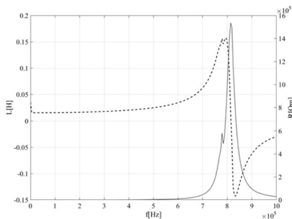
Fig. 8 The results of the measurement of inductance and resistance of the secondary winding as a function of frequency (secondary winding shorted, “-” – resistance, “- -” – inductance)
