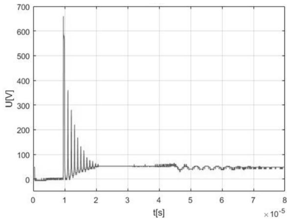
Fig. 15 The transistor voltage (drain-source) ( $U_{ds}$ ) in the HV triggering unit as a function of time – brake down on the spark gap
