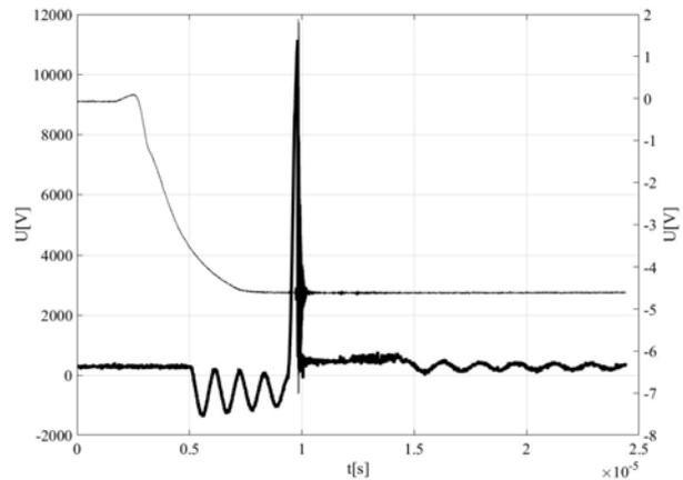
Fig. 18 The voltage sequence at the HV trigger output ( $U_{wy}$ ) - complete discharge
