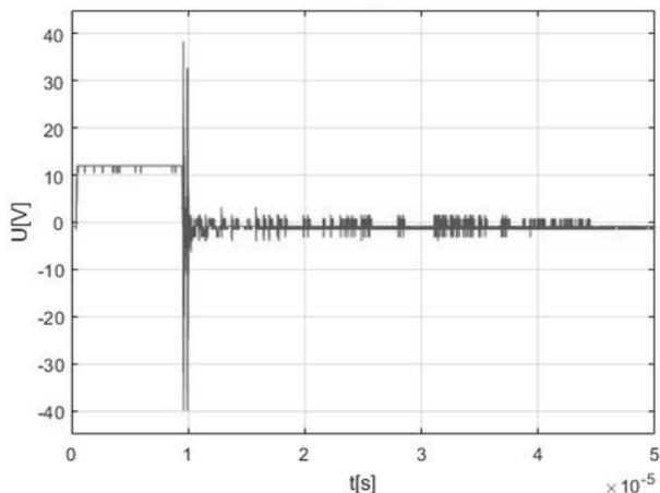
Fig. 16 The voltage waveform on the gate of the transistor ( $U_{gs}$ ) as a function of time - brake down on the spark gap
