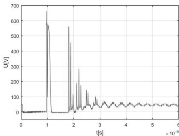
Fig. 11 Voltage waveform ( $U_{ds}$ ) on the transistor (drain-source) at the output of the HV triggering system as a function of time – no brake down on the spark gap
