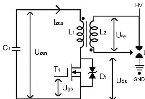
Fig. 2 The basic circuit diagram of the HV trigger; where: C1 - capacitor bank of total capacity 4000µF / 63V, L1, L2 - pulse transformer coils with turns ratio 10/480, T1 - chopping transistor, Dt - overvoltage protection, Is - controlled three-electrode spark gap.
