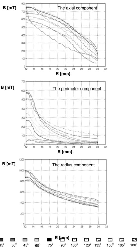
Fig.6. The course of the components of the vector of electromagnetic induction for all the measurement angles – joint fig.4, arrangement 1.
