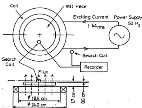
Fig. 1a. The examples of measuring the electromagnetic field: with the use of concentrically placed coils.
