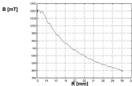
Fig.9c. The course of the components of the vector of electromagnetic induction for the selected measuring angle the radius component angles  $75^{\circ}$ .
