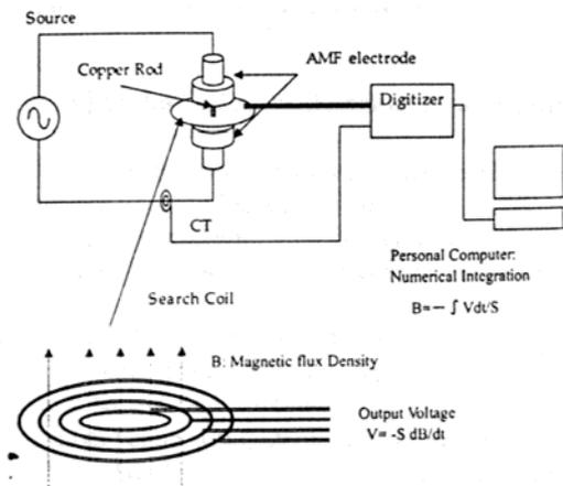
Fig. 1b. The examples of measuring the electromagnetic field with the use of the so called measuring probe
