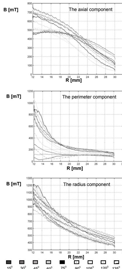
Fig.8: The course of the components of the vector of electromagnetic induction for all the measurement angles – joint fig.4, arrangement 2.
