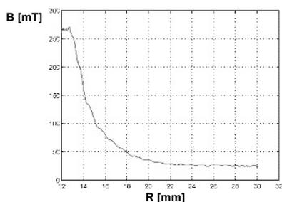
Fig.7b. The course of the components of the vector of electromagnetic induction for the selected measuring angle the perimeter component angles  $75^{\circ}$ .
