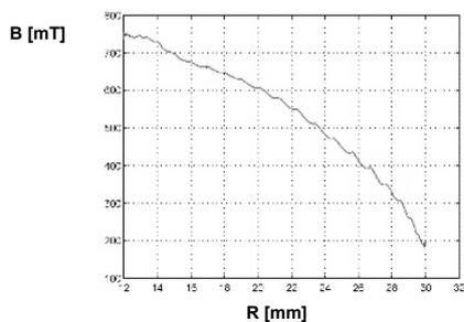
Fig.7a. The course of the components of the vector of electromagnetic induction for the selected measuring angle the axial component angles  $45^{\circ}$ .
