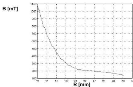
Fig.9b. The course of the components of the vector of electromagnetic induction for the selected measuring angle the perimeter component angles  $45^{\circ}$ .
