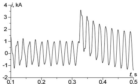
Fig.4. Transient current at the start of the line
