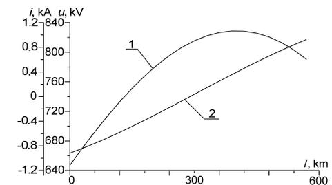
Fig.3. Spatial voltage (1) and current (2) waveforms along the line for the time  $t = 0.007$  s.
