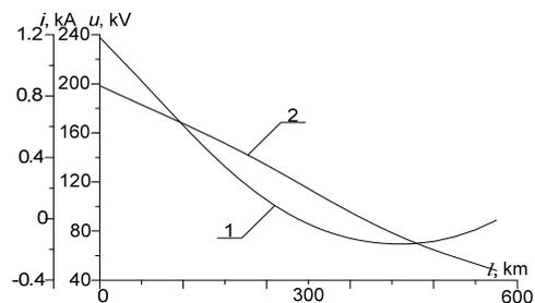
Fig.2. Spatial voltage (1) and current (2) waveforms along the line for the time  $t = 0.002$  s.
