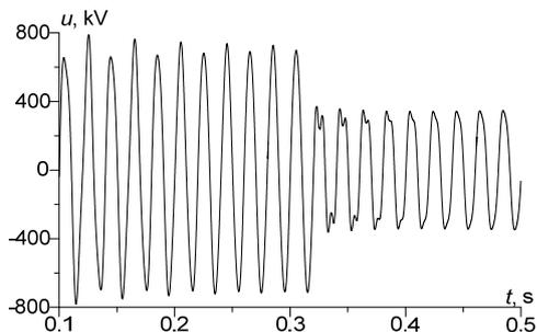
Fig.5. Transient voltage mid-line
