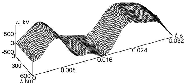
Fig.6. Temporal-spatial voltage waveform across the line for  $t \in [0; 0,032]$  s.
