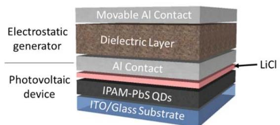
Fig. 1. Device Structure of the hybrid energy scavenger composed of a solution-processed photovoltaic structure (lower part) and an electrostatic generator (upper part).
