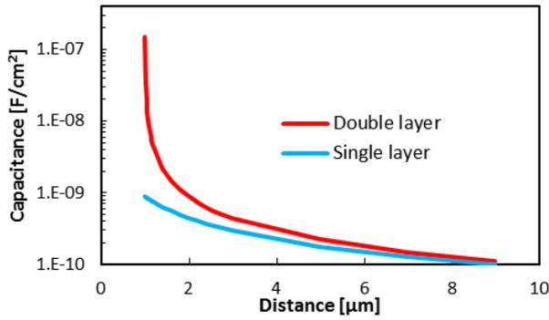
Fig. 3. Capacitance variation versus distance of the electrodes for two configurations.
