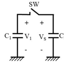
Fig. 5. Equivalent circuit diagram of the energy harvesting device
