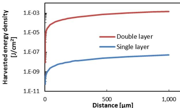
Fig. 4. Calculated harvested energy density versus the distance of the electrodes in single-layer and double-layer configurations. Both structures are supplied with a similar voltage source ( $V_0 = 341$  mV) at the initial state of the conversion cycle.
