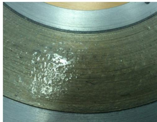
Fig.4. Fragment of stator core roll made of amorphous strip.
