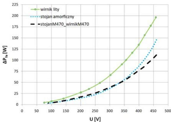
Fig.10. Comparison of iron losses vs. supply voltage at idle run, frequency 50 Hz
