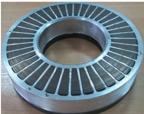
Fig.2. Cage rotor of disk-type induction motor; rotor is made of M470-50A strip, cage bars and both end-rings are visible.
