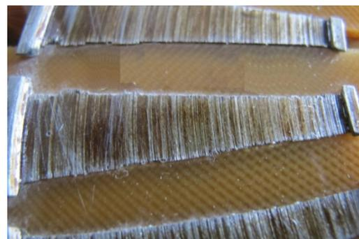
Fig.5. Fragment of stator core made of amorphous strip - after electro-erosion machining.
