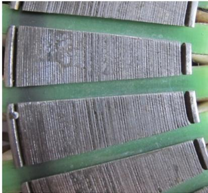
Fig.1. Fragment of stator core made of M470-50A strip - after electro-erosion machining.
