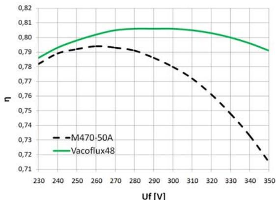
Fig.6. Efficiency vs. supply voltage at constant frequency 50 Hz for disk-type induction motor rated at 1.5 kW; strip M470-50A and strip Vacoflux48\_0.35mm.
