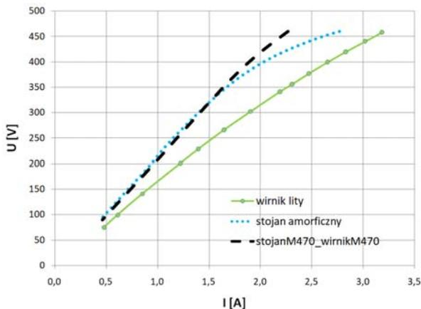
Fig.9. Comparison of magnetizing current vs. supply voltage
