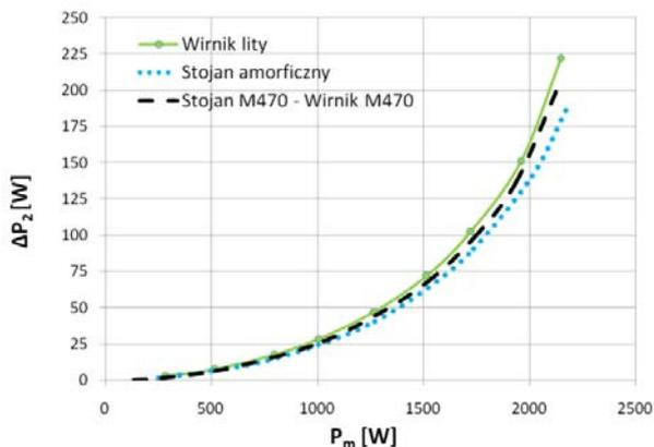
Fig.14. Comparison of rotor losses vs. load power (power at shaft) for different design variants.
