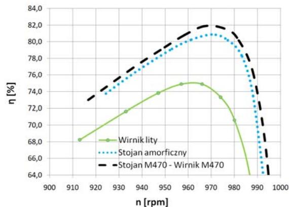
Fig.12. Efficiency coefficient  $\eta$  vs. rotational speed (slip) curves for different motor models, sinusoidal supply 400V, 50Hz.
