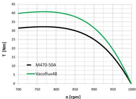
Fig.7. Torque at shaft vs. rotational speed for disk-type induction motor rated at 1.5 kW; strip M470-50A and strip Vacoflux48\_0.35mm.
