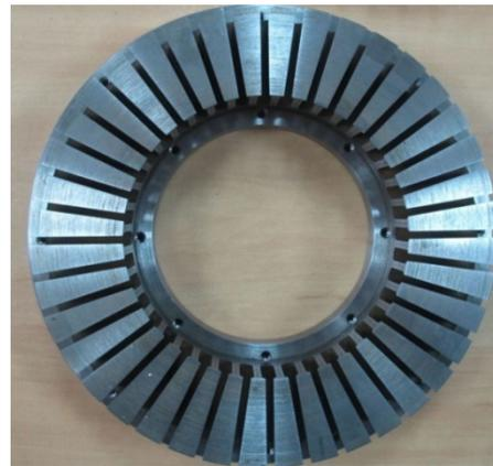
Fig.3. Rotor cage made of solid steel
