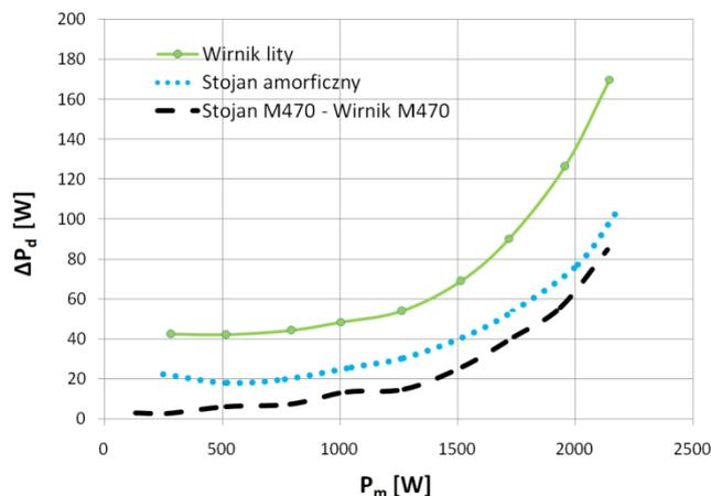
Fig.15. Comparison of remaining additional losses vs. load power (power at shaft) for different design variants.
