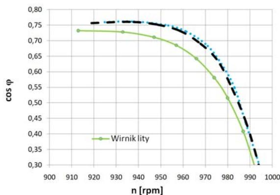
Fig.13. Power factor  $\cos\phi$  vs. rotational speed (slip) curves for different motor models, sinusoidal supply 400V, 50Hz.
