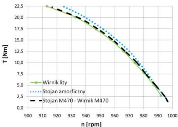
Fig.11. Torque vs. speed curves for different motor models, sinusoidal supply 400V, 50Hz.
