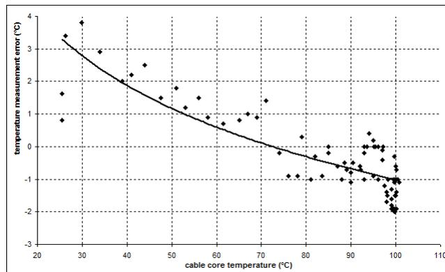
Fig.6. Absolute error in cable core temperature calculation
