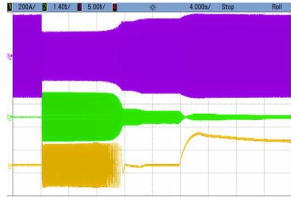
Fig.8. Start-up procedure of motor of machines set: 1 – current of excitation circuit, 2 - stator current, 3 - phase-to-phase voltage at the switchgear station
