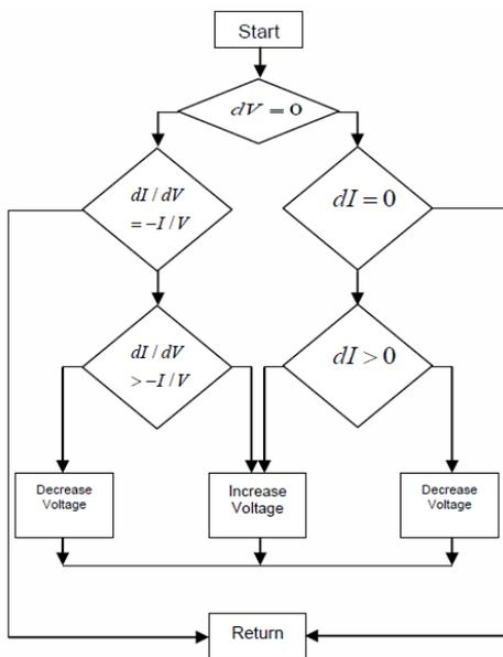
Figure 4: Incremental Conductance.
