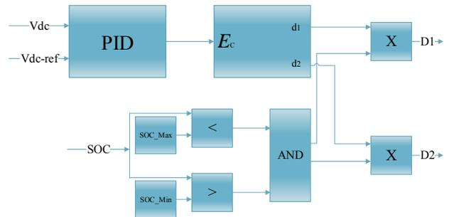
Figure 7: Control of the DC-DC bidirectional converter.
