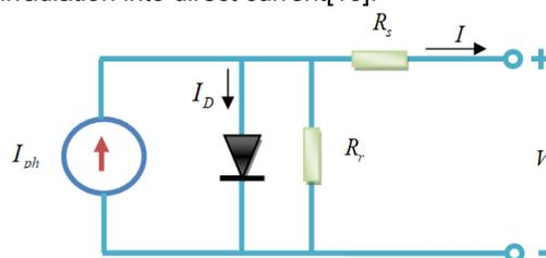
Figure 2: PV module equivalent circuit.
