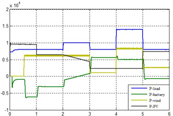
Figure 15: Wind-PV-Battery-Load Hybrid Power
