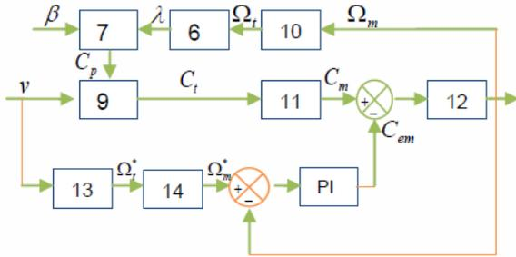
Figure 6: Direct speed control.
