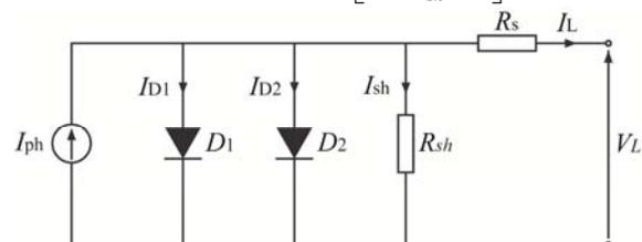
Fig. 1. Double diode model.
