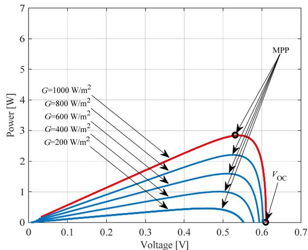
Fig. 4. The  $P$ - $V$  characteristics at varying irradiance.
