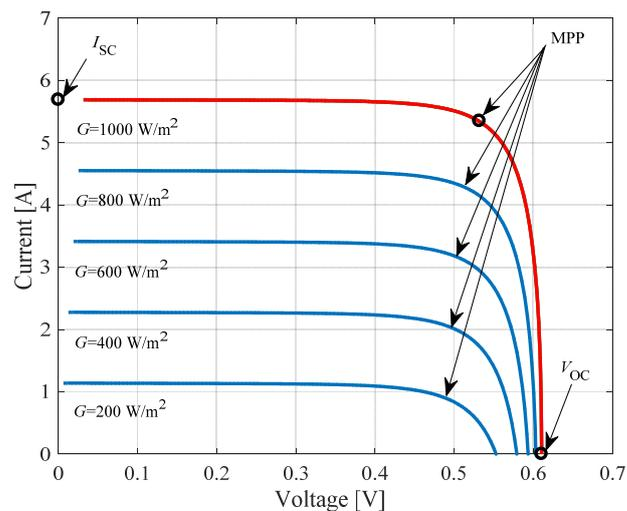
Fig. 3. The  $I$ - $V$  characteristics at varying irradiance.
