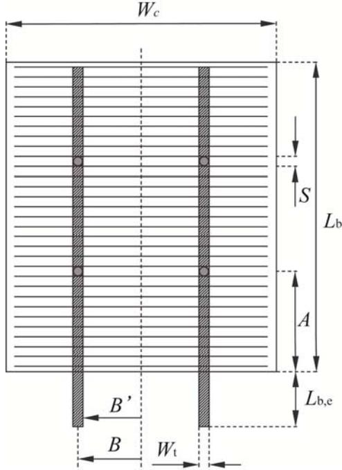
Fig. 2. An H-grid metallization pattern of solar cell.
