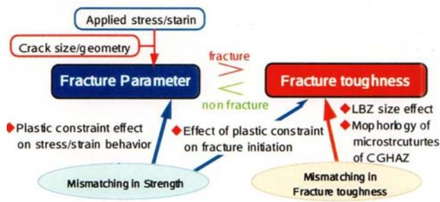
Fig. 3. Effect of mismatching on fracture-mechanics approach
