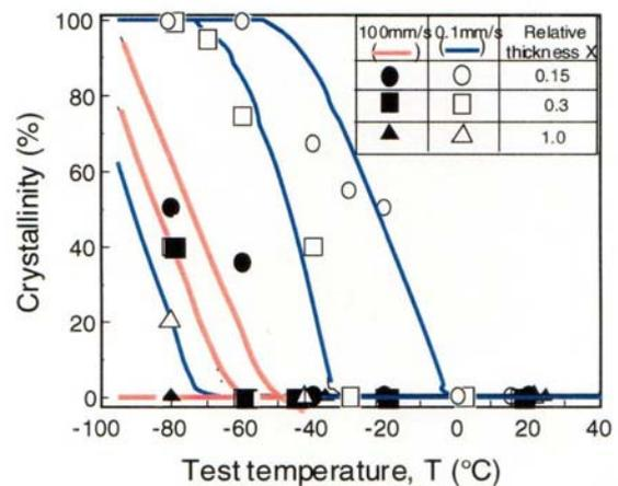
Fig. 8. Comparison of ductile-to-brittle transition behavior in undermatched joints.
