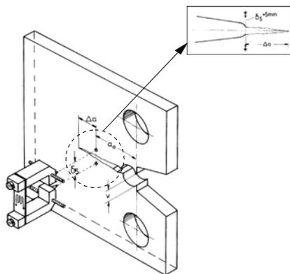
Fig. 6. Direct measurement of CTOD values at crack tip of fracture mechanics specimen
