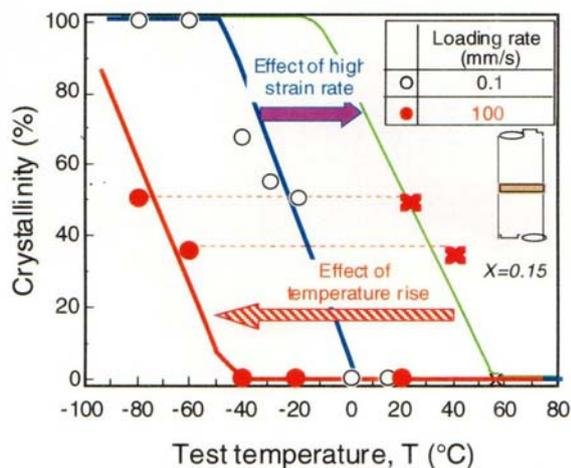
Fig. 9. Explanation of shift of ductile-to-brittle transition temperature in undermatched joints.
