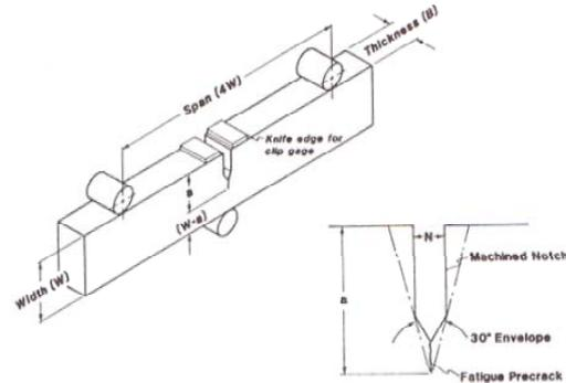
Fig. 4. Three-point bending CTOD test specimen.
