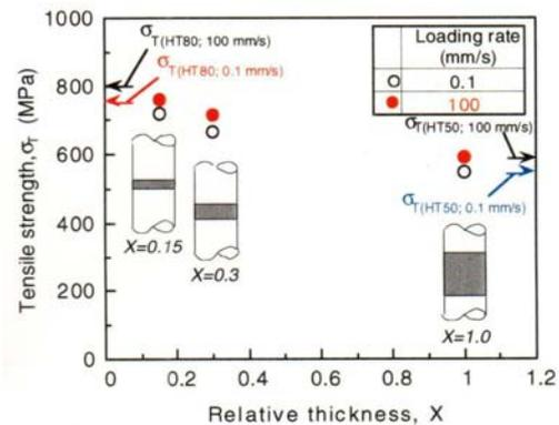
Fig. 7 Relationship between tensile strength and relative thickness in undermatched joints.
