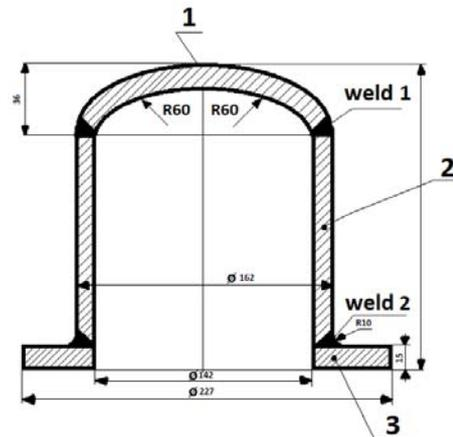
Fig. 1. Pressure vessel of prototype of Stirling engine operated as a hot cylinder with torispherical head, welded together with two undermached welds.
