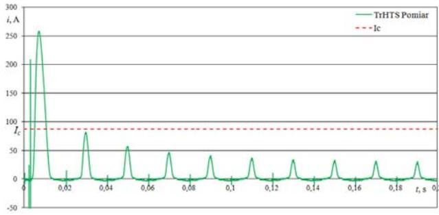
Fig. 5. The inrush current waveform of an 13.8 kVA HTS transformer
