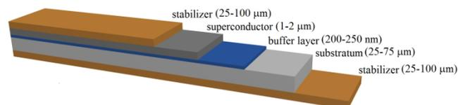
Fig. 3. General idea of 2G HTS cable structure [2]
