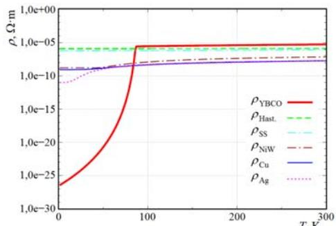
Fig. 9. The dependence of the resistivity of individual layers of the HTS tape on the temperature [5]
