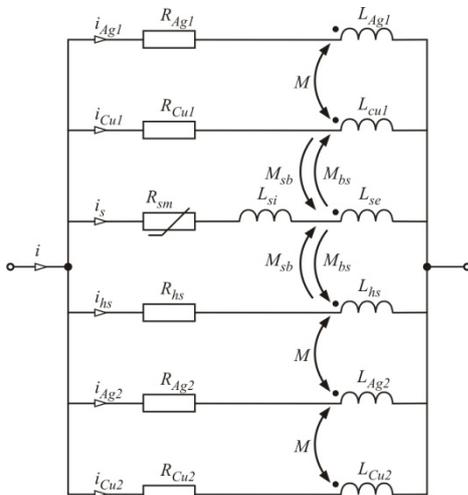
Fig. 7. Substitute scheme of the SCS4050 tape [3]
