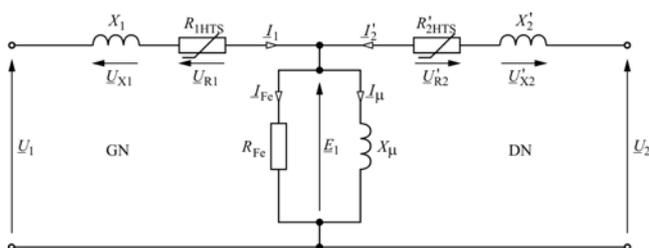
Fig. 1. Substitute diagram of the HTS transformer
