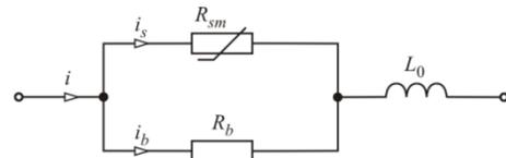
Fig. 8. A simplified diagram of the HTS transformer winding
