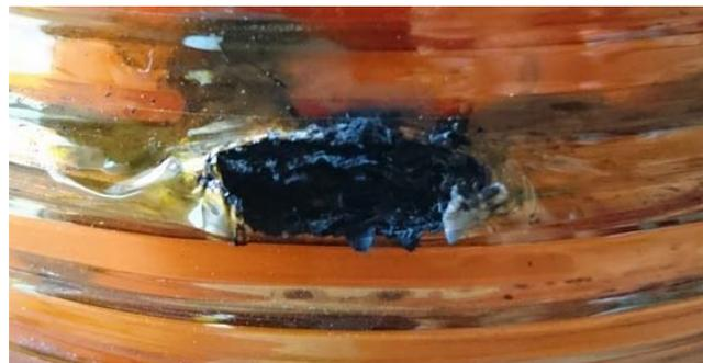
Fig. 4. Thermal damage of the upper voltage winding of an 13.8 kVA HTS transformer
