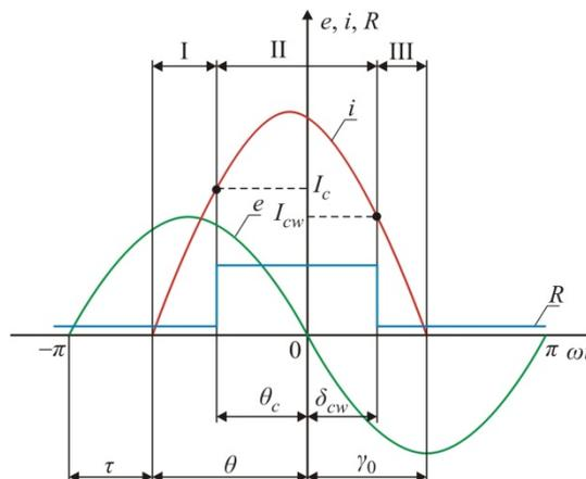
Fig. 10. The course of the inrush current impulse and changes in resistance of the HTS transformer winding during its duration and the power supply voltage;  $R$  – resistance of the superconductor transformer winding,  $e$  – supply voltage,  $i$  – one-way current pulse of the superconductor transformer,  $I_c$  – critical current of the transformer winding,  $I_{cw}$  – current at which the winding returns to the superconducting state
