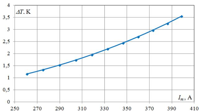
Fig. 11. Increase of the temperature of the primary winding of the HTS transformer for various peaks of the inrush current impulse [8]
