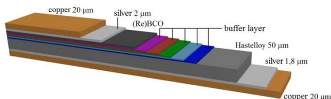
Fig. 2. Structure of the 2G HTS cable from SuperPower Inc. [1]
