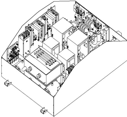
Fig.3. View of the circuit breaker DCU-800MNL after removing the top cover
