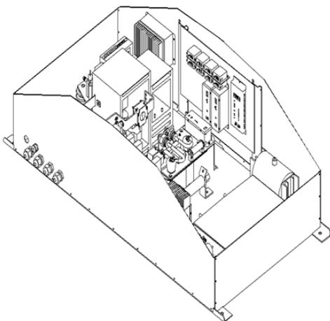
Fig.1. View circuit breaker DCU-800MNL after removing the top cover
