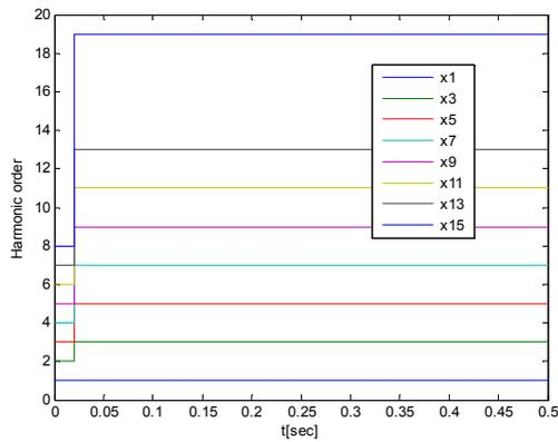
Fig.12. Estimated States' order in adaptive Kalman filter for the 3<sup>rd</sup> input signal.
