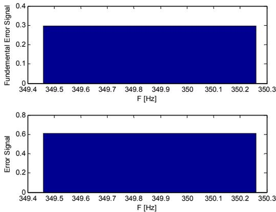
Fig.3. FFT of the Fundamental error and Error signals when Kalman filter modelled all the input signal harmonic components except the 7<sup>th</sup> order harmonic.
