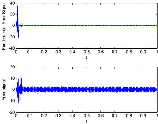
Fig.11. Fundamental error and Error signals of the adaptive Kalman filter for the 3<sup>rd</sup> input signal.
