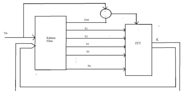
Fig.6. Block diagram of the adaptive Kalman filter.
