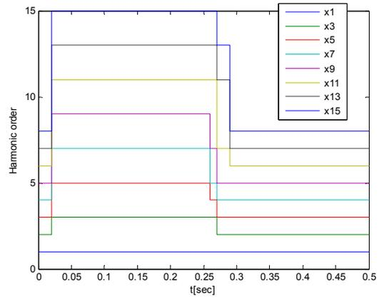
Fig.15. Estimated States' order in adaptive Kalman filter for the 4<sup>th</sup> input signal.
