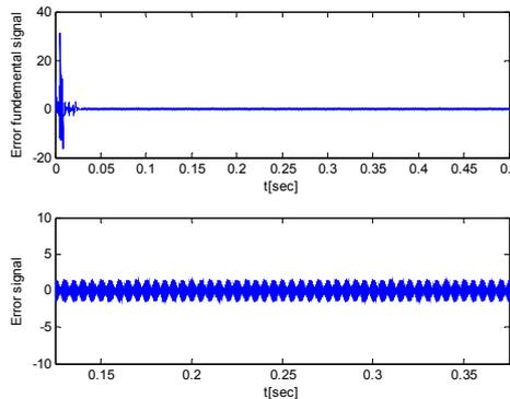
Fig.9. Fundamental error and Error signals of the adaptive Kalman filter for the 2<sup>nd</sup> input signal.
