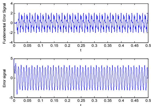
Fig.4. Fundamental error and Error signals when Kalman filter modelled all the input signal harmonic components except the 2<sup>nd</sup> and 7<sup>th</sup> order harmonics.
