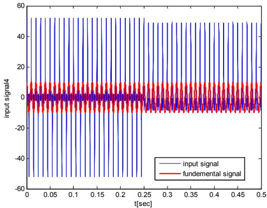
Fig.13. Input signal that has variable order harmonics.
