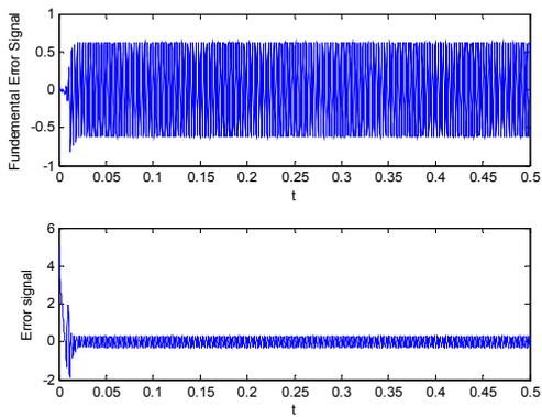
Fig.2. Fundamental error and Error signals when Kalman filter modelled all the input signal harmonic components except the 7<sup>th</sup> order harmonic.
