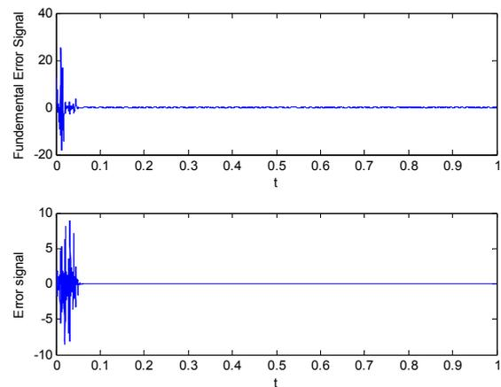
Fig.17. Fundamental error and Error signals of the adaptive Kalman filter for the 5<sup>th</sup> input signal.
