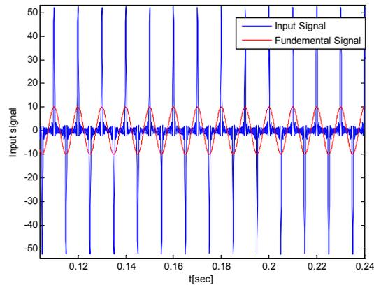
Fig.16. 5<sup>th</sup> Input signal SNR equals 30.
