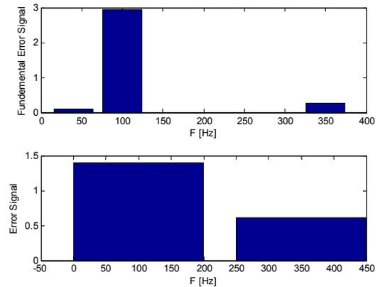
Fig.5. FFT of the Fundamental error and Error signals when Kalman filter modelled all the input signal harmonic components except the 2<sup>nd</sup> and 7<sup>th</sup> order harmonics.
