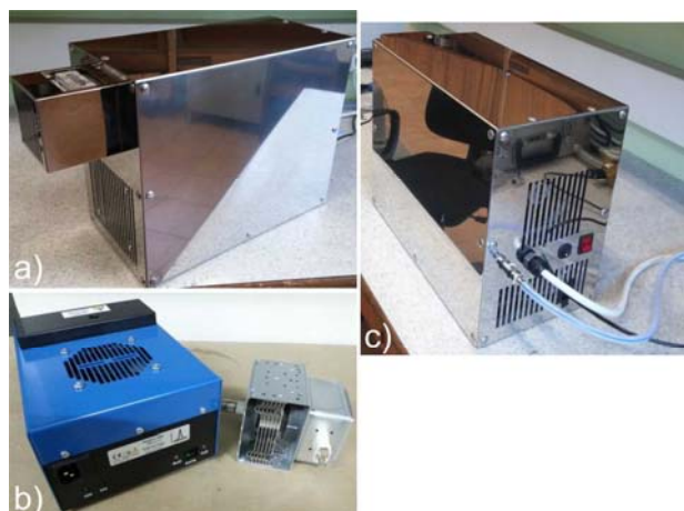
Fig.8. Photos of the novel compact microwave plasma device for surface treatment: (a) front view, (b) built-in high voltage power supply and magnetron, (c) rear view
