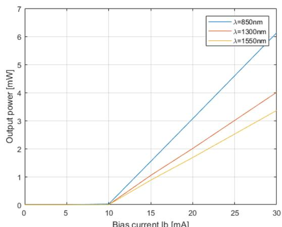
Fig. 3. Optical power dependencies on the input bias current for different wavelengths
