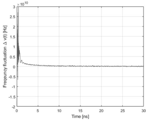
Fig.67 Central lasing frequency fluctuations during the transient
