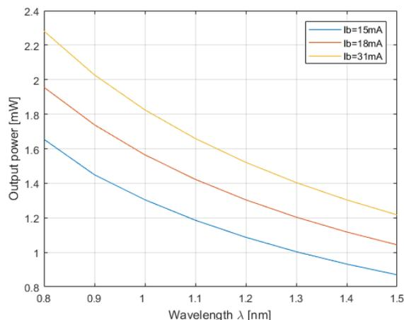
Fig. 2. Optical power dependencies on the central lasing wavelength for different bias currents
