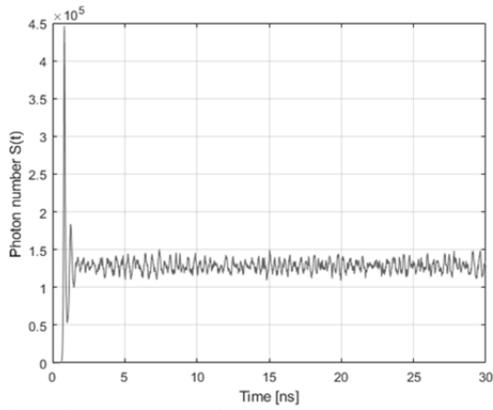
Fig. 4 Photon number fluctuations during the transient
