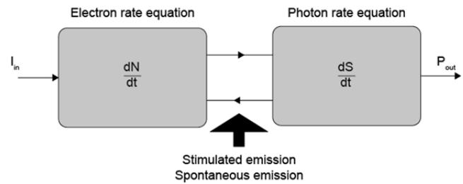
Fig.1. The single-mode laser model expressed by the rate equation
