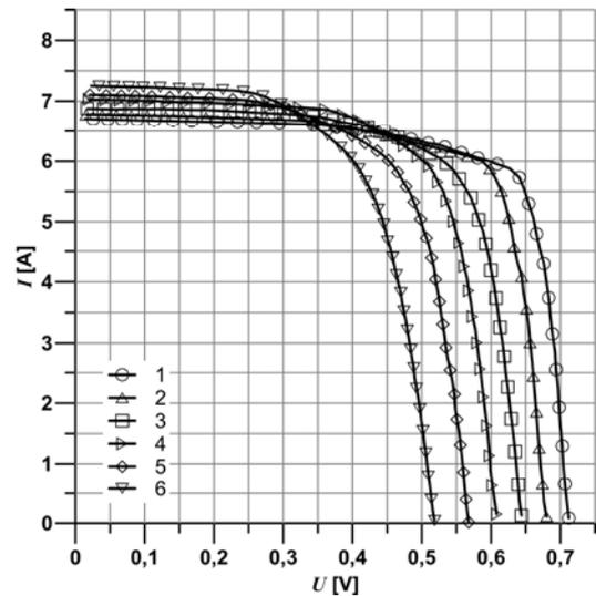
Fig.3. Dependences  $I = f(U)$  for sample 2 recorded for different operating temperatures: 1 –  $-20^\circ\text{C}$ , 2 –  $0^\circ\text{C}$ , 3 –  $25^\circ\text{C}$ , 4 –  $50^\circ\text{C}$ , 5 –  $75^\circ\text{C}$ , 6 –  $100^\circ\text{C}$
