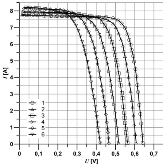
Fig.2. Dependences  $I = f(U)$  for sample 1 recorded for different operating temperatures: 1 –  $-20^\circ\text{C}$ , 2 –  $0^\circ\text{C}$ , 3 –  $25^\circ\text{C}$ , 4 –  $50^\circ\text{C}$ , 5 –  $75^\circ\text{C}$ , 6 –  $100^\circ\text{C}$
