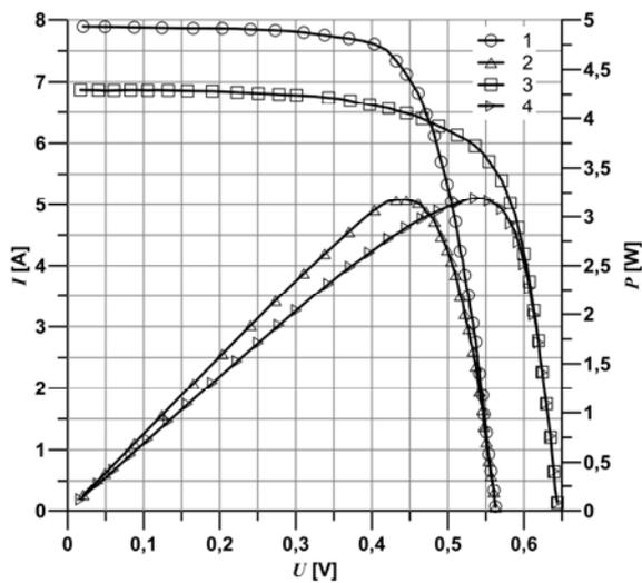
Fig.1. Dependences  $I = f(U)$  and  $P = f(U)$  for different types of c-Si PV cells (I-V and P-V curves respectively): 1, 2 – conventional cell, 3, 4 – HIT-IBC cell
