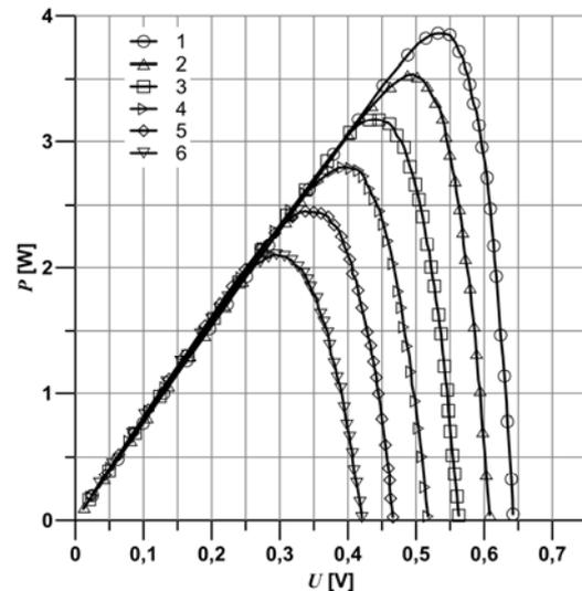
Fig.4. Dependences  $P = f(U)$  for sample 1 recorded for different operating temperatures: 1 –  $-20^\circ\text{C}$ , 2 –  $0^\circ\text{C}$ , 3 –  $25^\circ\text{C}$ , 4 –  $50^\circ\text{C}$ , 5 –  $75^\circ\text{C}$ , 6 –  $100^\circ\text{C}$
