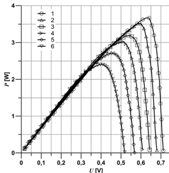
Fig.5. Dependences  $P = f(U)$  for sample 2 recorded for different operating temperatures: 1 –  $-20^\circ\text{C}$ , 2 –  $0^\circ\text{C}$ , 3 –  $25^\circ\text{C}$ , 4 –  $50^\circ\text{C}$ , 5 –  $75^\circ\text{C}$ , 6 –  $100^\circ\text{C}$
