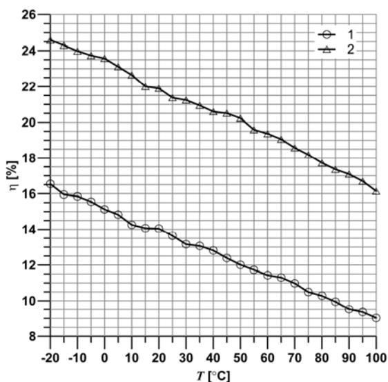
Fig.6. Dependences of the solar cells efficiency  $\eta$  vs. ambient temperature  $T$ , recorded for tested samples: 1 – conventional cell (sample 1), 2 – HIT-IBC cell (sample 2)
