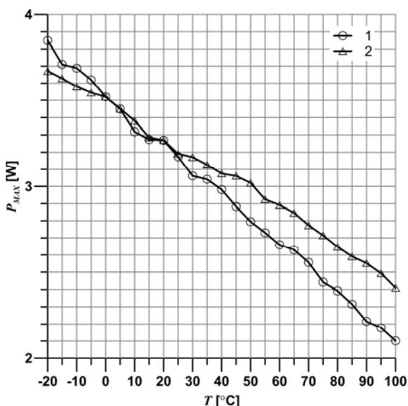
Fig.7. Dependences of the solar cells maximum power  $P_{MAX}$  vs. ambient temperature  $T$ , recorded for tested samples: 1 – conventional cell (sample 1), 2 – HIT-IBC cell (sample 2)
