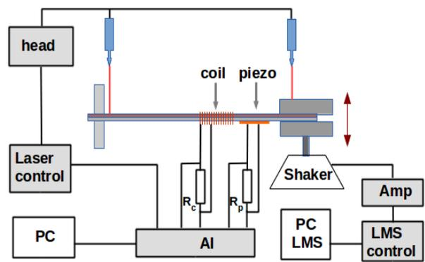
Fig. 2. The experimental stand scheme.
