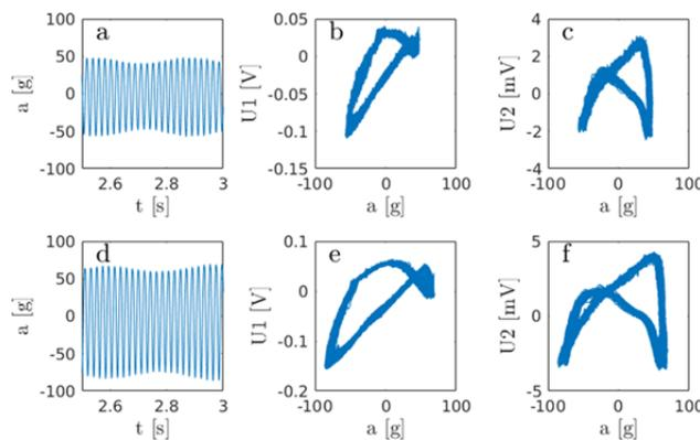
Figure 5. The acceleration measured by laser and the voltage hysteresis loops of both subsystems for different level of external forcing:  $a = 0.8$  g (a, b, c) and  $a = 1.5$  g (d, e, f).
