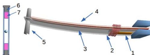
fig. 1. The pipe (left) and double beam structure (right) with piezo (1) and electromagnetic (2) transducers. (3) – alumina beam, (4) magnetostrictive beam, (5) – alumina pipe as tip mass. (6) – closing cap, (7) – flexible bumper (top).
