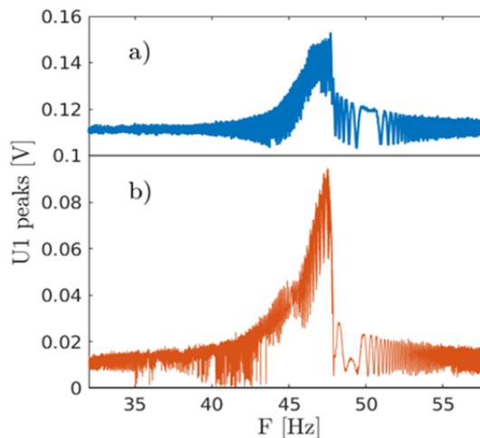
Fig. 4. Voltage output response of piezoelectric ( $U_1$ ) subsystem without the moving ball for frequency sweep and amplitude of the excitation  $a = 0.8$  g (a) and  $a = 1.5$  g (b).
