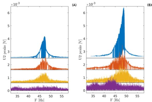
Fig. 3. Voltage output response of magnetostrictive subsystem ( $U_2$ ) for frequency sweep and amplitude of the excitation  $a = 0.8$  g (A) and  $a = 1.5$  g (B). The blue color corresponds to no moving mass, orange - M1, yellow - M2 and purple - M1+M2, respectively.
