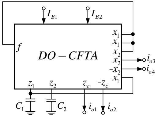
Fig. 5. Proposed current-mode quadrature oscillator
