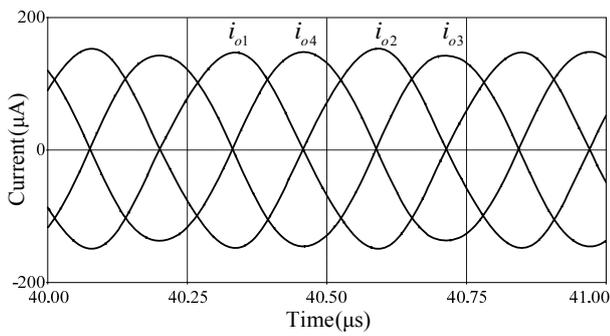
Fig. 8. Quadrature output waveforms in steady state
