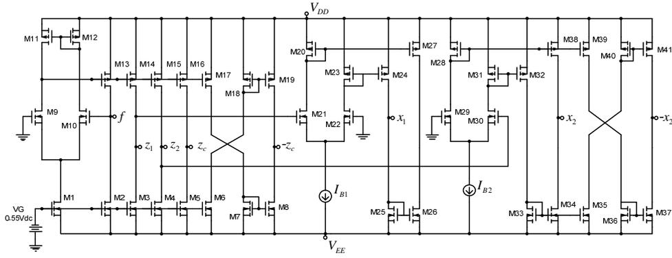
Fig. 3. Internal construction of DO-CFTA
