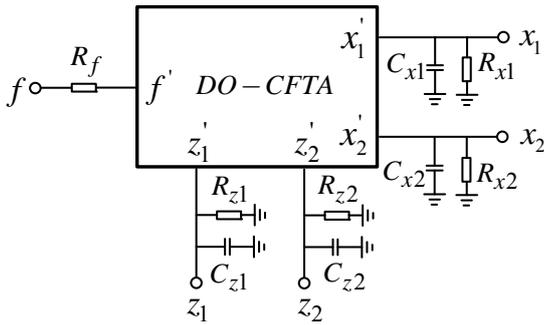
Fig. 6: Parasitic resistances and capacitances of DO-CFTA
