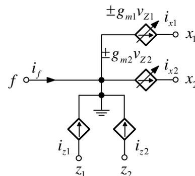
Fig. 2. Equivalent circuit of DO-CFTA
