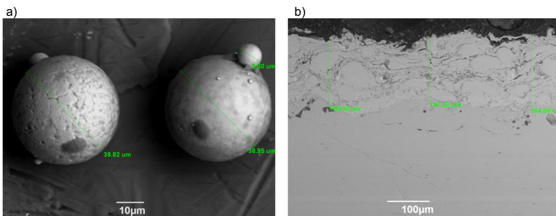
Fig.3. SEM images of NiCrBSi alloy powder particles (a) and the cross-section of the powder coating deposited by MPS on a steel substrate (b) External view of MP-004 manufactured by E. O. Paton EWI, Ukraine (a) and the process of micro-plasma deposition of wire coating on the surface of a cylindrical shaft (b) at the experimental site for micro-plasma surface treatment at D. Serikbayev EKSTU.
