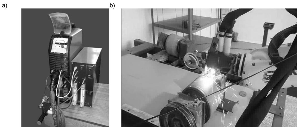
Fig.1. External view of MP-004 manufactured by E. O. Paton EWI, Ukraine (a) and the process of micro-plasma deposition of wire coating on the surface of a cylindrical shaft (b) at the experimental site for micro-plasma surface treatment at D. Serikbayev EKSTU.
