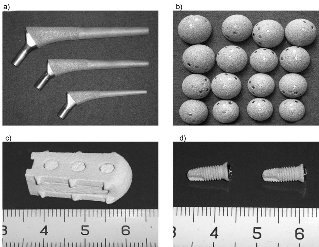
Fig.2. Examples of products with biocompatible coating deposited by microplasma spraying at the E. O. Paton EWI: components of hip implants (a), (b); implant for interbody spondylosyndesis (c); dental implants (d).
