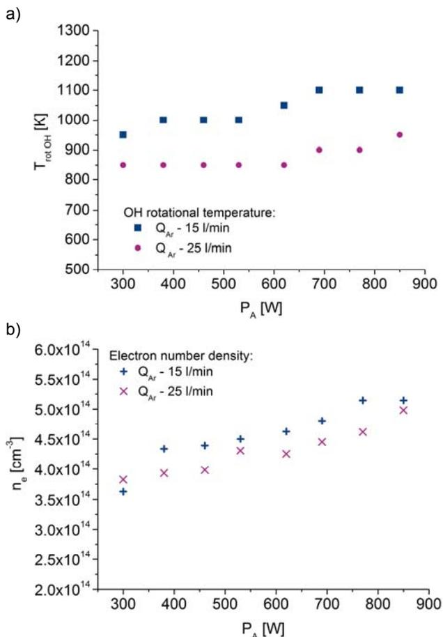
Fig.5. Rotational temperatures of OH radicals (a) and electron number density (b) as a function of microwave absorbed power  $P_A$  (for Ar flow rate  $Q_{Ar}$  - 15 and 25 l/min).
