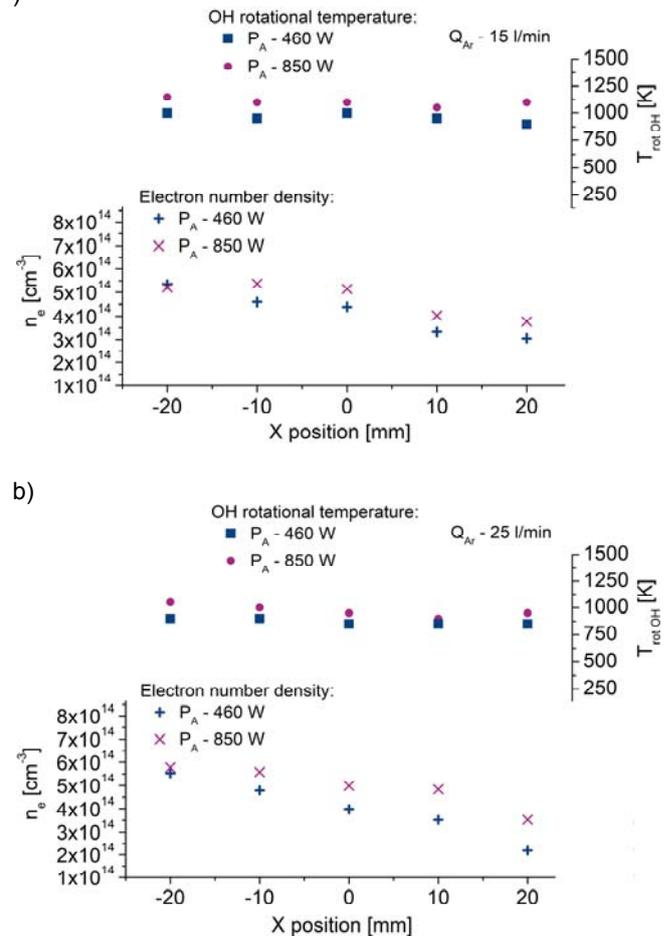
Fig.4. Rotational temperatures of OH radicals and electron number density as a function of X position in plasma for microwave absorbed power  $P_A$  460 and 850 W and Ar flow rate  $Q_{Ar}$  15 l/min
