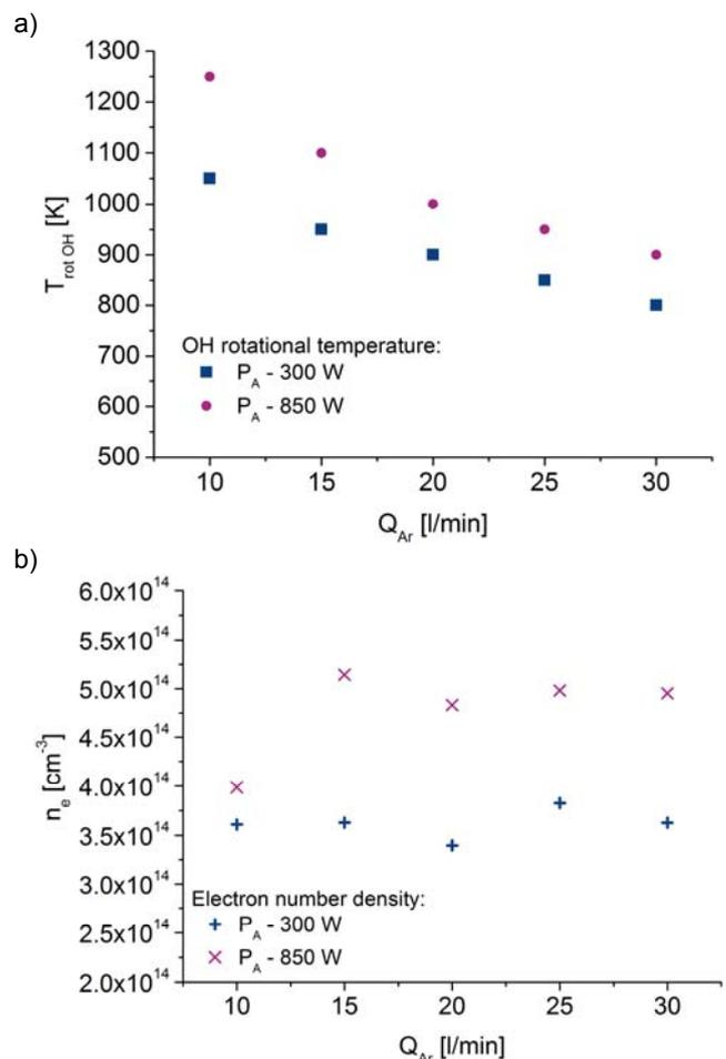
Fig.6. Rotational temperatures of OH radicals (a) and electron number density (b) as a function of Ar flow rate  $Q_{Ar}$  (for microwave absorbed power  $P_A$  - 300 and 850 W).
