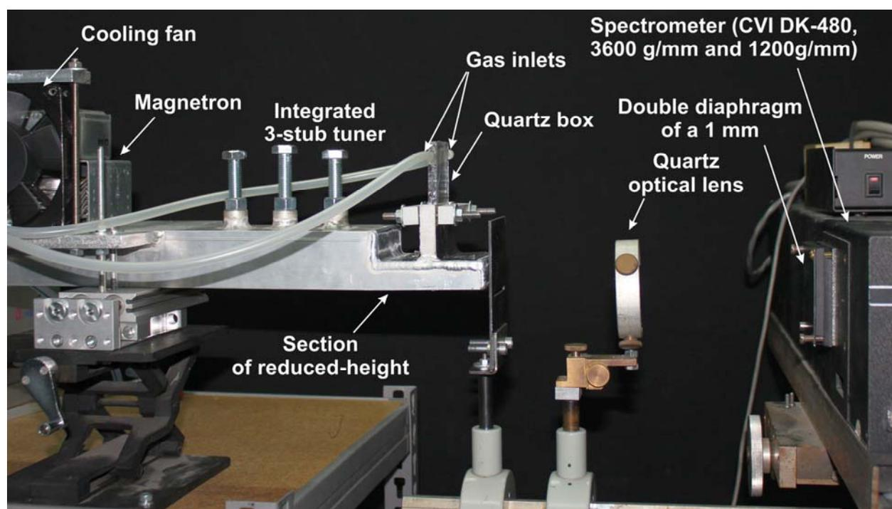
Fig. 1. The experimental setup for spectroscopic study of argon microwave atmospheric pressure plasma-sheet.
