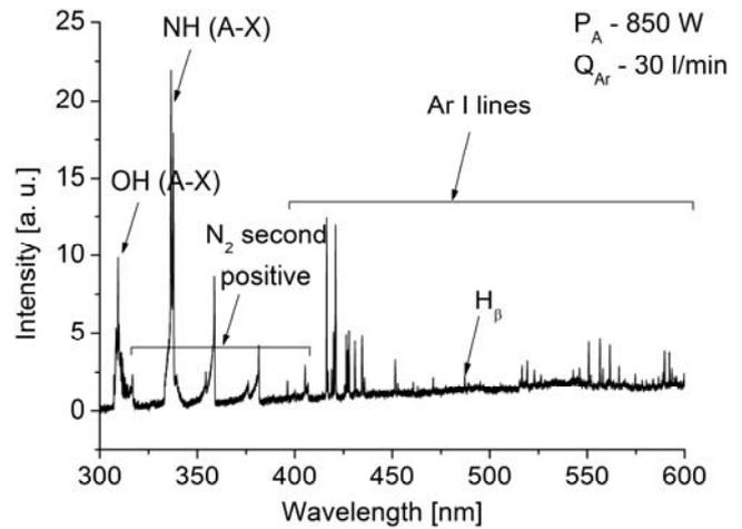
Fig. 3. Measured emission spectrum of argon plasma ( $P_A = 850$  W, Ar flow rate  $Q_{Ar} = 30$  l/min, X position - 0mm)
