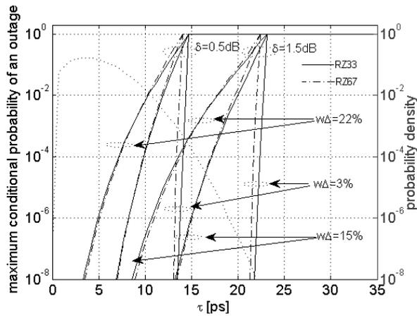
Fig. 4. Conditional outage probability (solid and dash-dot lines) versus momentary DGD backgrounded by probability density of DGD in a typical 500km long single mode fiber (dotted line).
