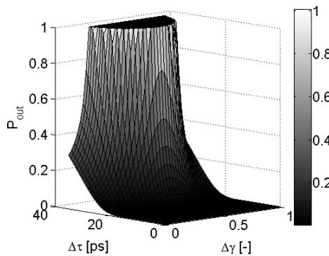
Fig.3. Conditional probability of an outage versus momentary DGD and power split ratio.
