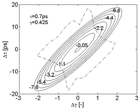
Fig.2. Contour of the tolerance area to errors of compensator control. In the background: isolines of exemplary logarithmic normalized probability density of the errors.
