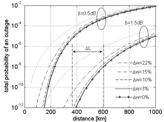
Fig. 5. Total probability of an outage versus length of an optical fiber.
