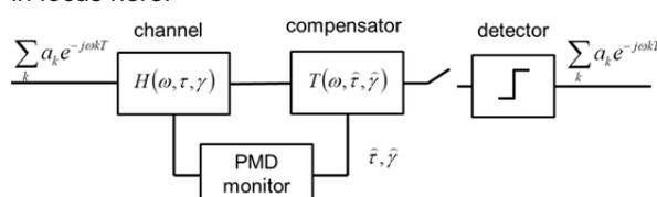
Fig.1. First order PMD compensation with the use of an electronic Feedforward Equalizer (FFE).
