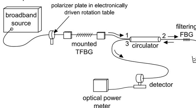
Fig.4. The scheme of proposed interrogation setup for demodulation of input light polarization plane angle
