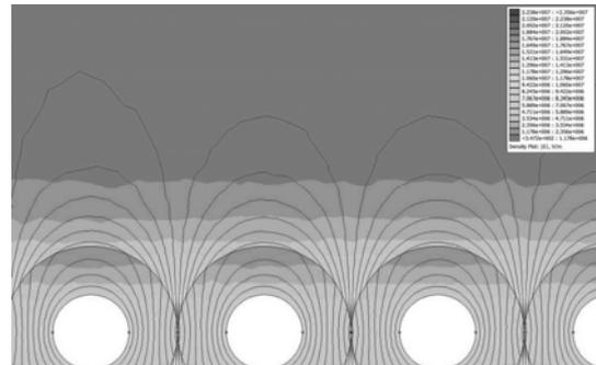
Fig. 4. Distribution of electric field intensity in bifilar winding with a solid chassis (voltage 10 kV, wire cross-section 1.0  $\text{mm}^2$ )
