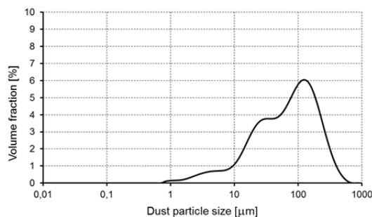
Fig. 2b. Volume distribution of dust particle size for B type dust
