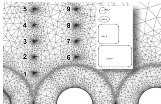
Fig. 5. Placement of dust particles around the bifilar winding during simulation
