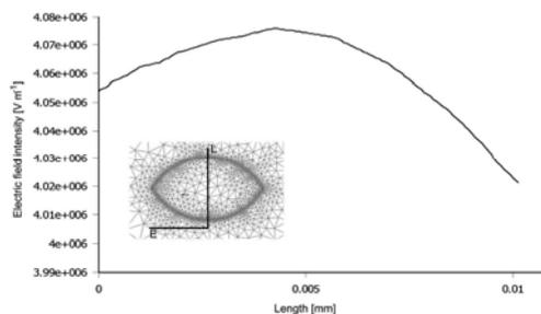
Fig. 7. Distribution of the electric field intensity along the vertical axis of the ellipsoidal cross-section sample (point 1)
