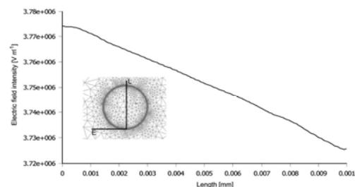
Fig. 6. Distribution of the electric field intensity along the vertical axis of the circular cross-section sample (point 1)
