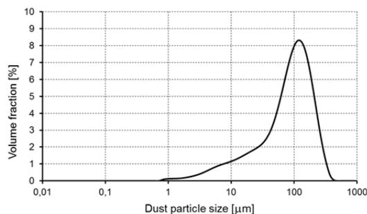
Fig. 2c. Volume distribution of dust particle size for C type dust
