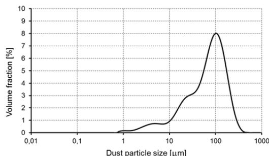
Fig. 2a. Volume distribution of dust particle size for A type dust
