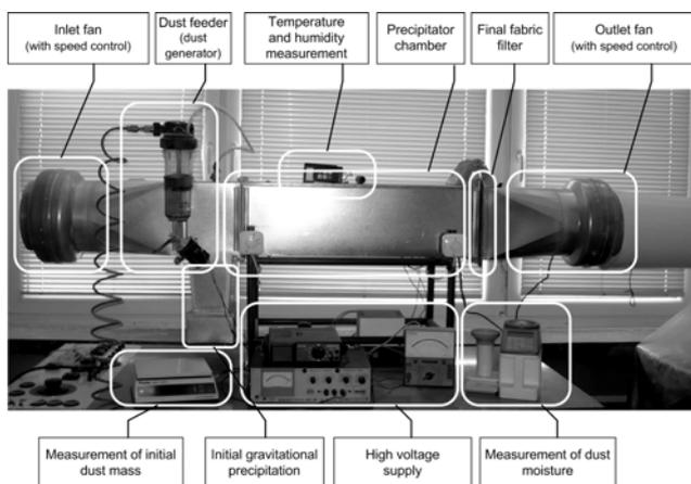
Fig. 1. View of bifilar filtration system
