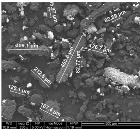
Fig. 3a. View of dust particles at 250x magnification
