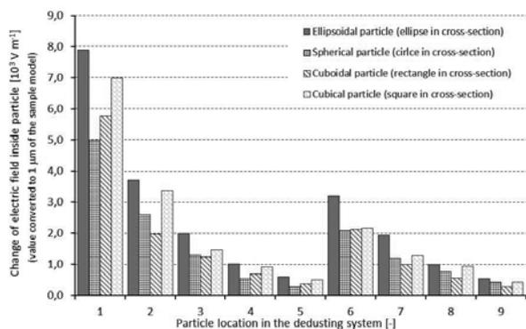
Fig. 8. Change of electric field intensity ( $\cdot 10^3 \text{ V} \cdot \text{m}^{-1}$ ) inside particle for placement in the dedusting system converted to  $1 \mu\text{m}$  of the sample model
