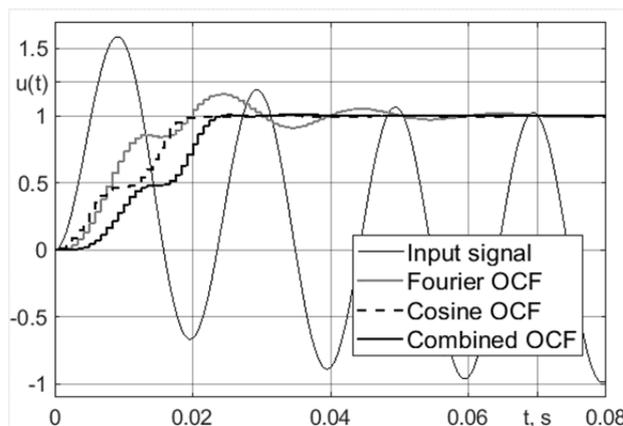
Fig. 5. The reaction of the OCF to a sinusoidal signal with an aperiodic component being contained in it
