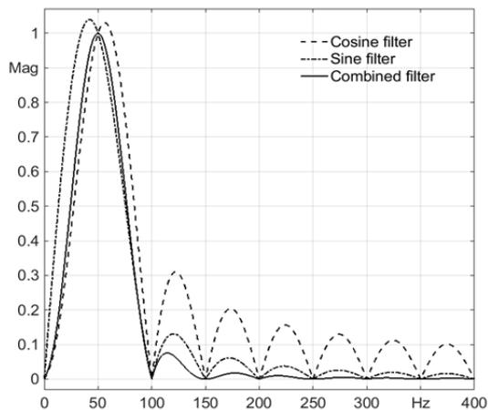
Fig. 2. The frequency responses of the filters configured for 50 Hz
