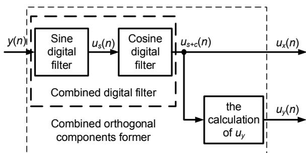
Fig. 1. Structural scheme of the combined OCF
