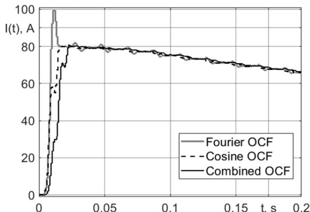
Fig. 7. The separation of the amplitude of the second harmonic in the inrush of the magnetizing current
