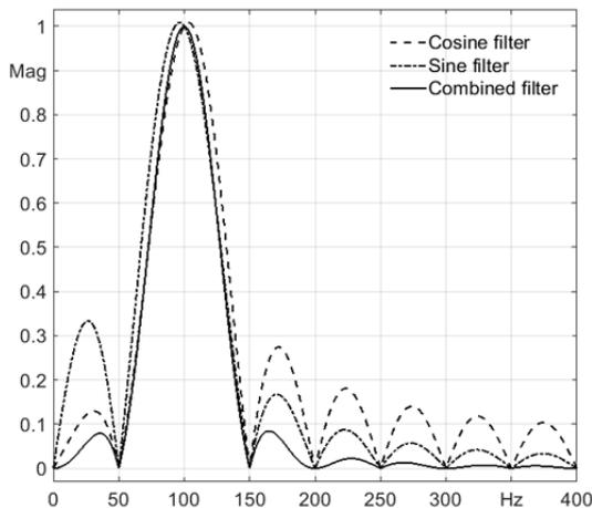
Fig. 3. The frequency response of filters configured to 100 Hz
