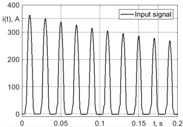
Fig. 6. The inrush of magnetizing current of one phase of a power transformer
