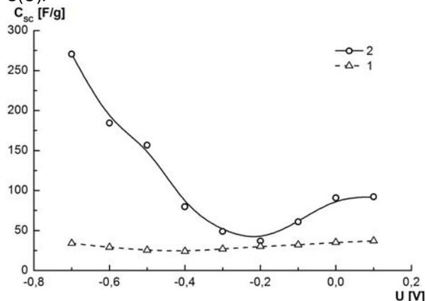
Fig. 5. Dependence of capacitance specific value  $C_{SC}$  on the constant bias voltage for the initial activated carbon (1) and for activated carbon after 10 min ultrasonic influence (2)
