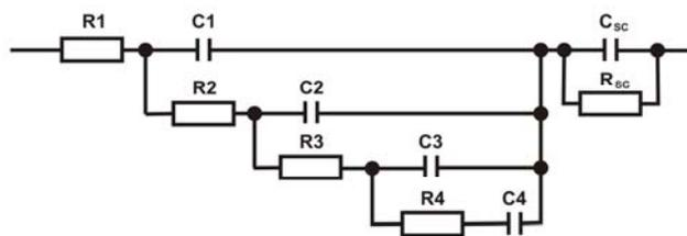
Fig. 4. Equivalent electrical circuit modelling the impedance hodographs for the initial and modified activated carbon
