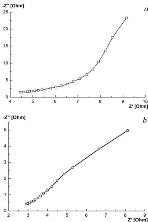
Fig. 3. Typical Nyquist diagrams for the initial (a) and modified (b) activated carbon
