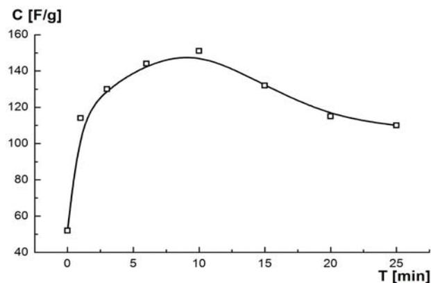
Fig. 1. Dependence of specific capacitance of activated carbon from the time of ultrasonic treatment
