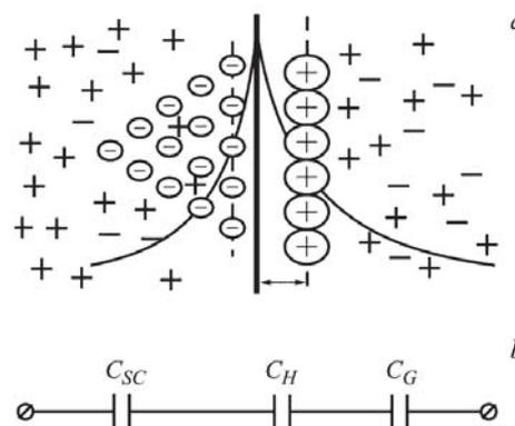
Fig. 2. Model of electric double layer for non-metallic electrodes (a) and the equivalent electrical circuit (b) [13]
