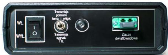
Fig. 8. Front panel of the transmitter block [own results]
