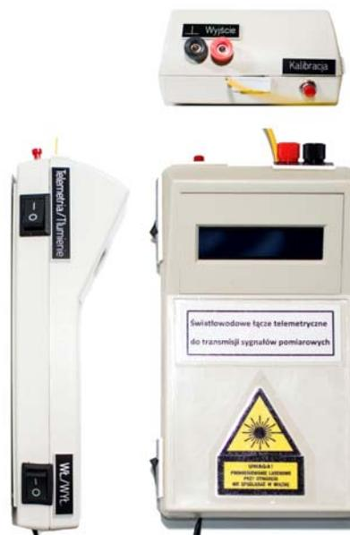
Fig. 11. Front panel of the receiver block RX and its side and top view [own results]
