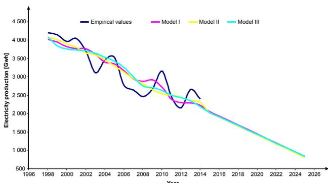
Fig. 7. Empirical values and forecast of electrical energy production in utility hydropower plants
