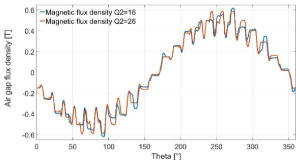
Fig. 5: Radial air-gap flux density distribution with respect to angular position
