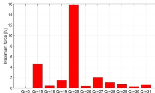
Fig. 13 Maximum force with variable rotor slit number
