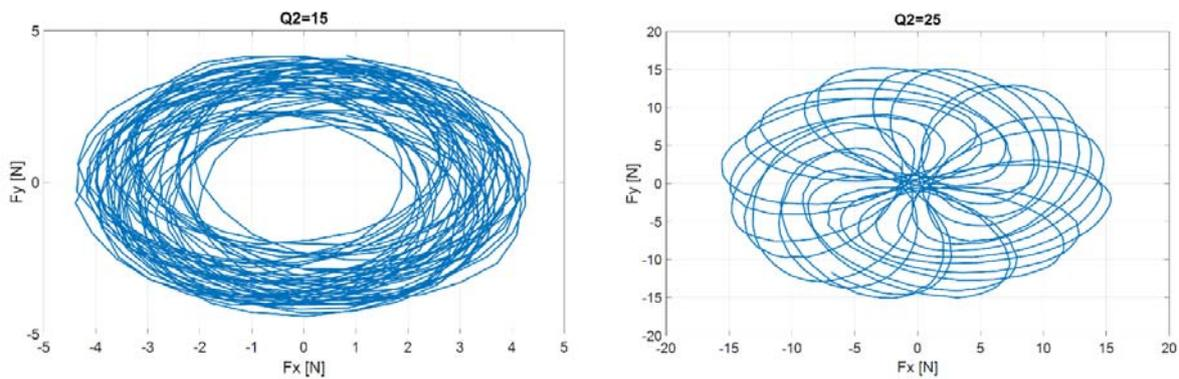
Fig. 14: The trace of forces in x and in y direction with odd number of rotor slits 15 and 25
