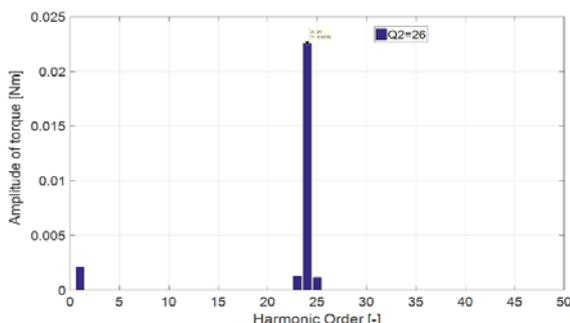
Fig. 10: Harmonic spectrum of given torque, where motor operate under no load, Q2=26
