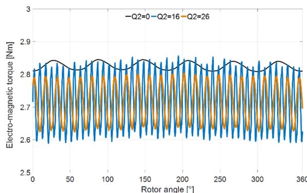
Fig. 7: Electromagnetic torque vs. rotor mechanical angle where number of rotor slits is Q2=0, 16, 26
