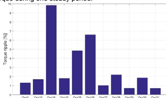
Fig. 8: Magnitude of torque ripple with variable rotor slit number
