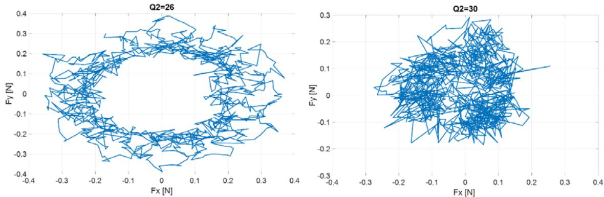
Fig. 15: The trace of forces in x and in y direction with even number of rotor slits 26 and 30
