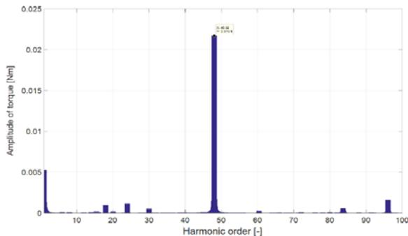
Fig. 11: Harmonic spectrum of given torque, where motor operate under no-load, Q2=16
