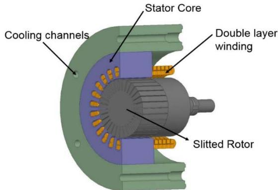
Fig. 1: 3D cross section of HSIM
