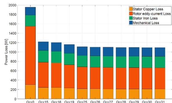
Fig. 3: Power losses in HSIM with different rotor slits
