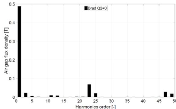
Fig. 9: Air gap flux density harmonic spectrum for smooth rotor, without rotor slits
