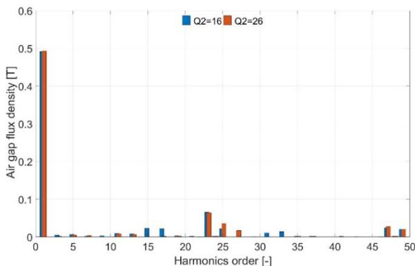
Fig. 6: Air gap flux density harmonic spectrum
