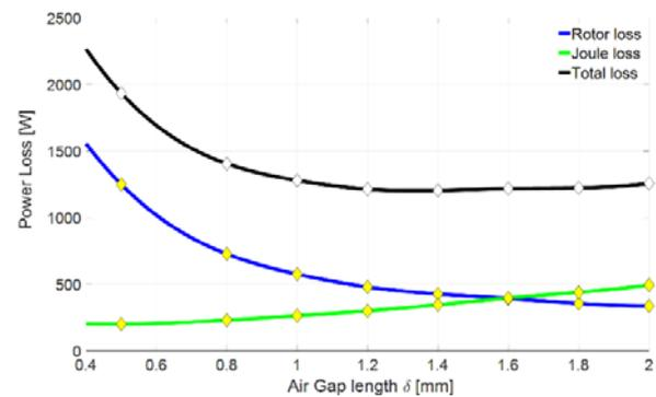
Fig. 2: Power loss division in HSIM with variable airgap
