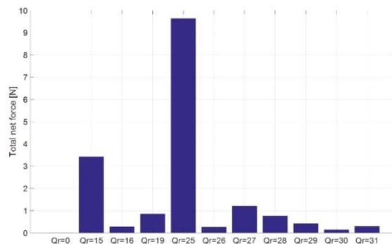
Fig. 12: total net force with variable rotor slit number
