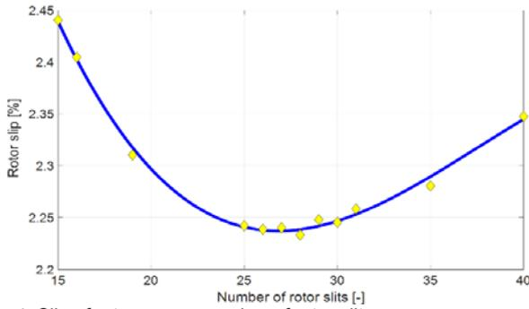
Fig. 4: Slip of rotor versus number of rotor slits
