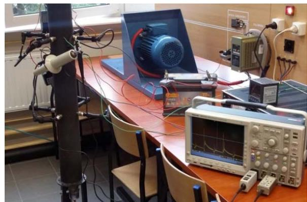
Fig.5. A setup to test ignition systems.
