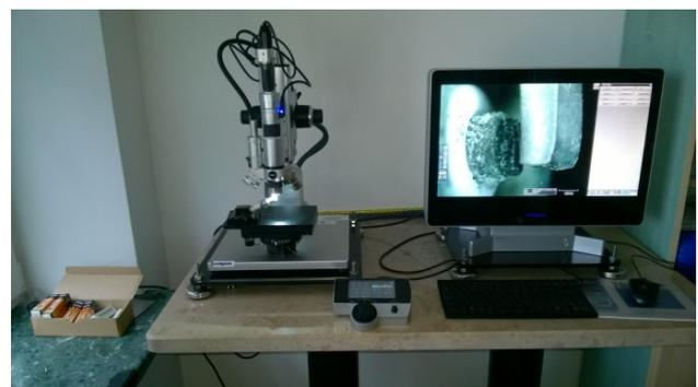
Fig 6. Microscope stand for the observation of electrode wear
