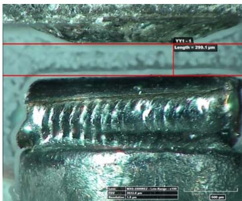
Fig. 8. The image of the gap between electrodes before the test
