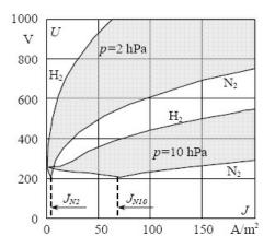
Fig.1. Electrical characteristics for DC glow discharge
