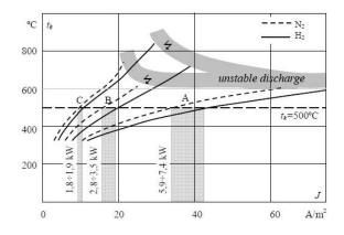
Fig. 3. Static characteristics of workload temperature in function of current density in insulated and non-insulated vacuum discharge chambers
