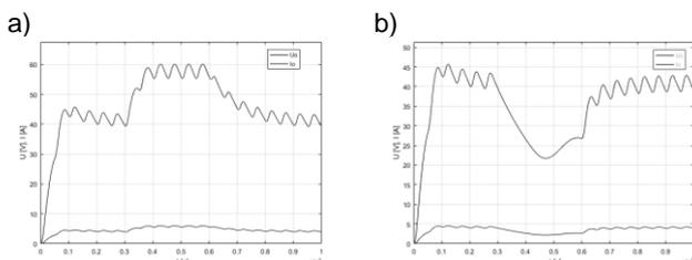
Fig. 13 Output voltage of FORWARD converter: a) with diode D<sub>2</sub> disturbances, b) with diode D<sub>2</sub> disturbance and clock path.
