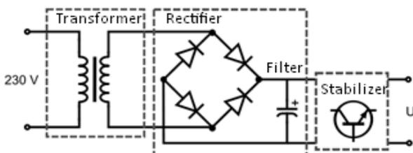
Fig. 1 Linear power supply diagram.
