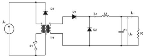
Fig. 4 Diagram of a FORWARD converter.
