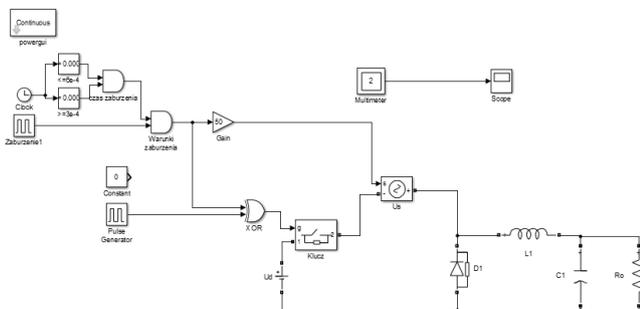
Fig. 5 Numerical model of BUCK type converter
