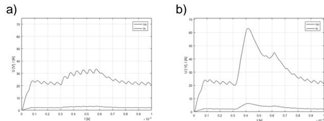
Fig. 9 Converter with disturbances: a) in front of diode D, b) in front of clock line.
