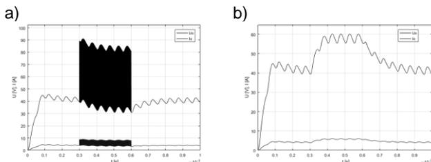
Fig. 12 Output voltage of FORWARD converter: a) with load disturbances R0, b) with L1C1 filter.
