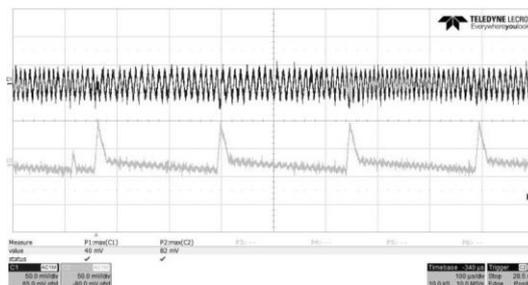
Fig. 17 Input and output voltages of the universal converter at a load current of 25 mA.
