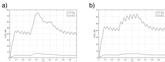
Fig. 14 Output voltage of FORWARD converter with transformer disturbances in: a) winding 1, b) winding 2.
