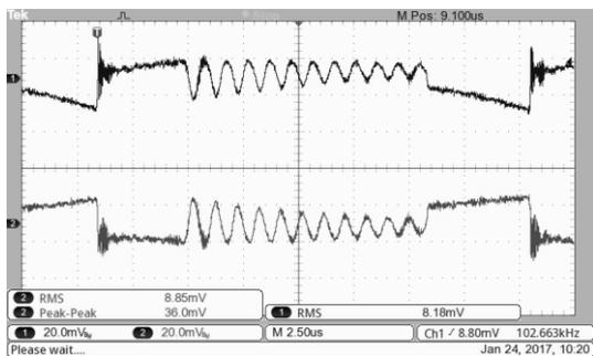
Fig. 20 Voltage reduction converter - work without disturbance.
